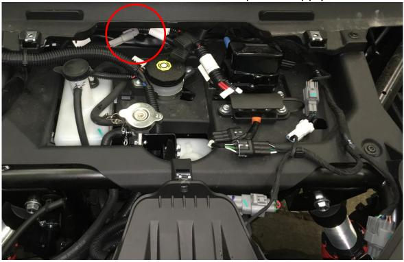
Drill the hole Ø 35 mm for heater harness to the plastic cover.
