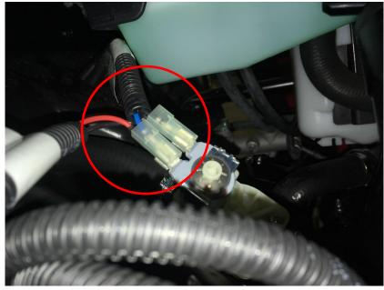
Connect the water pump harness with the water pump.
