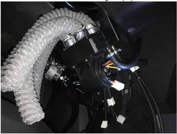
Drill two holes  $\emptyset$  55 mm to the dashboard for the heater air hoses
