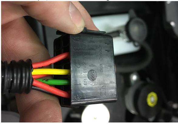
Connect the wiper/washer harness with the wiper/washer switch. Install the wiper/washer switch into the UTV dashboard.
