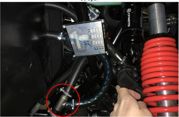
Connect the heating hoses using the bleeding valve together. Use tightening straps for fixing.
