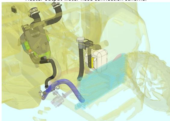
Connect the heater output water hose assembly to the bottom hose on the front cooler radiator.
