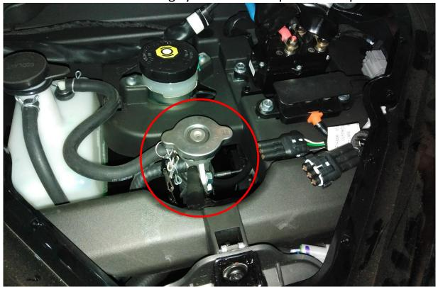
Dismantle two fixing screws on the radiator pressure cap and mount the washer tank holder with washer tank. Use the original screws.
