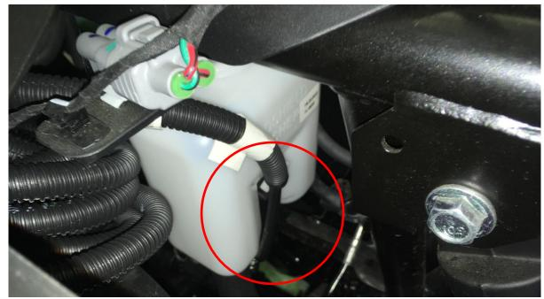
Route the wiper/washer harness through the prepared hole on dashboard.
