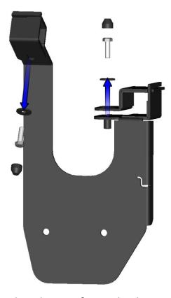
Remove the clamps from the heater holder.
