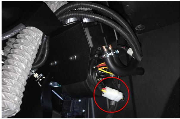
Route the front heater air hoses through the heater control panel holes.
