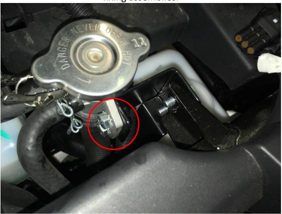
Connect the wiper/washer harness with the power supply harness.
