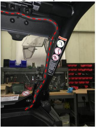
Connect the wiper/washer harness to the wiper motor.
