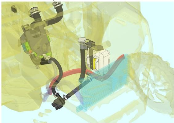
Connect the heater input water hose assembly to the upper hose on the front cooler radiator.
