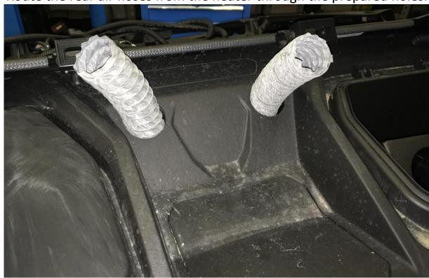
Cut the air hoses to correct length and insert the air vents onto the hoses. Fix the air vents with the hoses by included tightening straps. Press the air vents into the holes.
