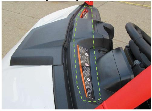
Install the original warning sticks onto the DFK front upper ledge. (View on installed front upper ledge)
