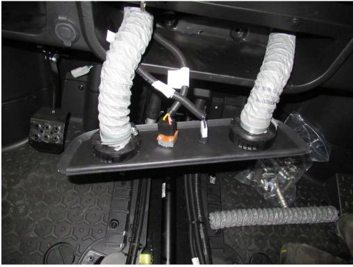
Place the cover onto the dashboard and fix the cover by included screws.
