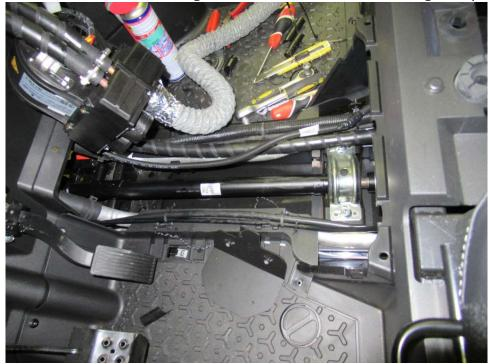
Install the el. valve and the water pump into the heater hose. Run the heater harness to the el. valve. Connect the heater harness with the el. valve and with the water pump.
