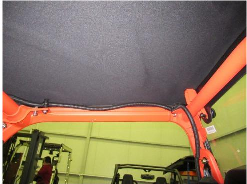
Run the wiper harness from the rear vehicle frame to the front panel.
