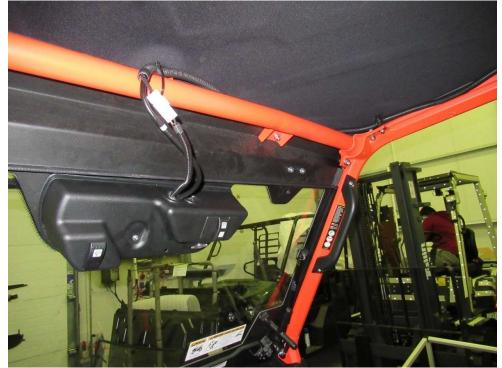
Install the wiper motor assembly onto the front window.
