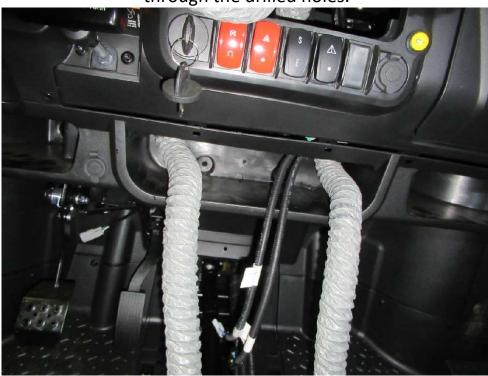
Connect the heater harness with the switches on the cover.
