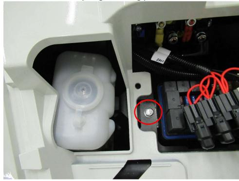
Connect the relay harness with the original electro-installation. Red wire with the +12V (red mark), black wire with the -12V (green mark).
