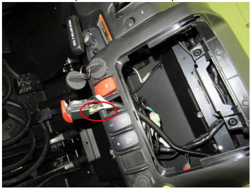
Insert the wiper harness into the inner dashboard space. Connect the harness with the washer tank.
