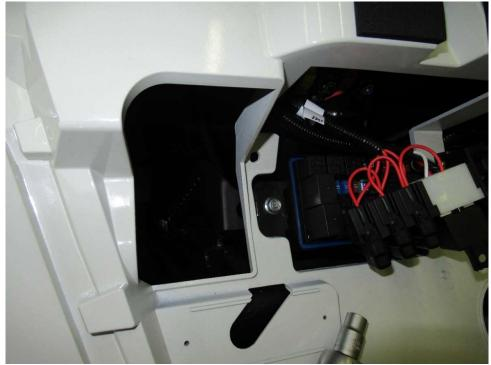
Install the relay assembly with the vehicle by original fixing point.
