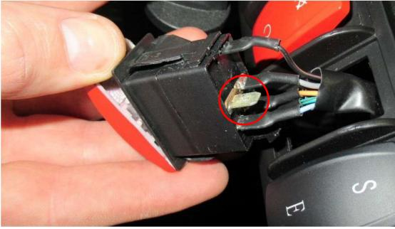
Connect the relay harness with the free pin on the switch. Push the switch back to the dashboard.
