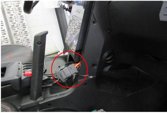
Push the wiper/washer switch to the dashboard.
