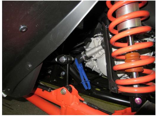
Secure the original engine cooling hose by clamps or pliers (not included).
