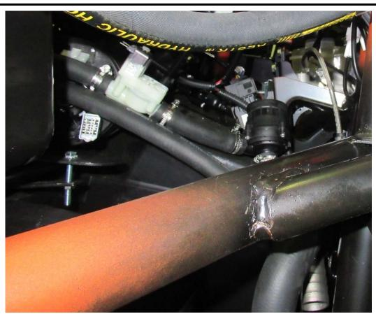
Slide on tightening ring onto the heater hose. Insert the "Y" tube into the heater hose. Secure the hose by the rings. Prepare both hoses like this.
