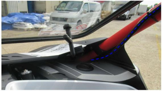
Fasten the wiper harness with included cable ties.
