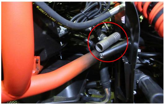
Cut the heater hose and slide on tightening rings onto the hose.
