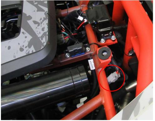
Connect the heater harness with the heater.
