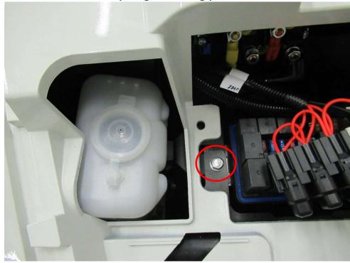
Connect the relay harness with the original electro-installation.
