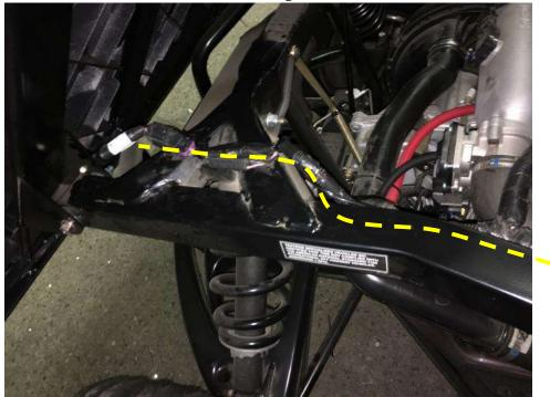
Open the original brake light harness (after the original connection) and connect brake light harness with the original brake light harness <u>RED/BLUE</u> wire by included connector. SEE NEXT PAGE
