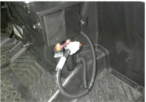
Connect the pump harness with the el. Valve. Connect the heater harness with the pump harness.
