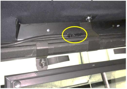
Run the work light harness from the wiper motor assembly to the work light. Connect the work light with the work light harness. 106
