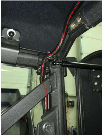
Run the washer harness from the washer tank to the front upper ledge.
