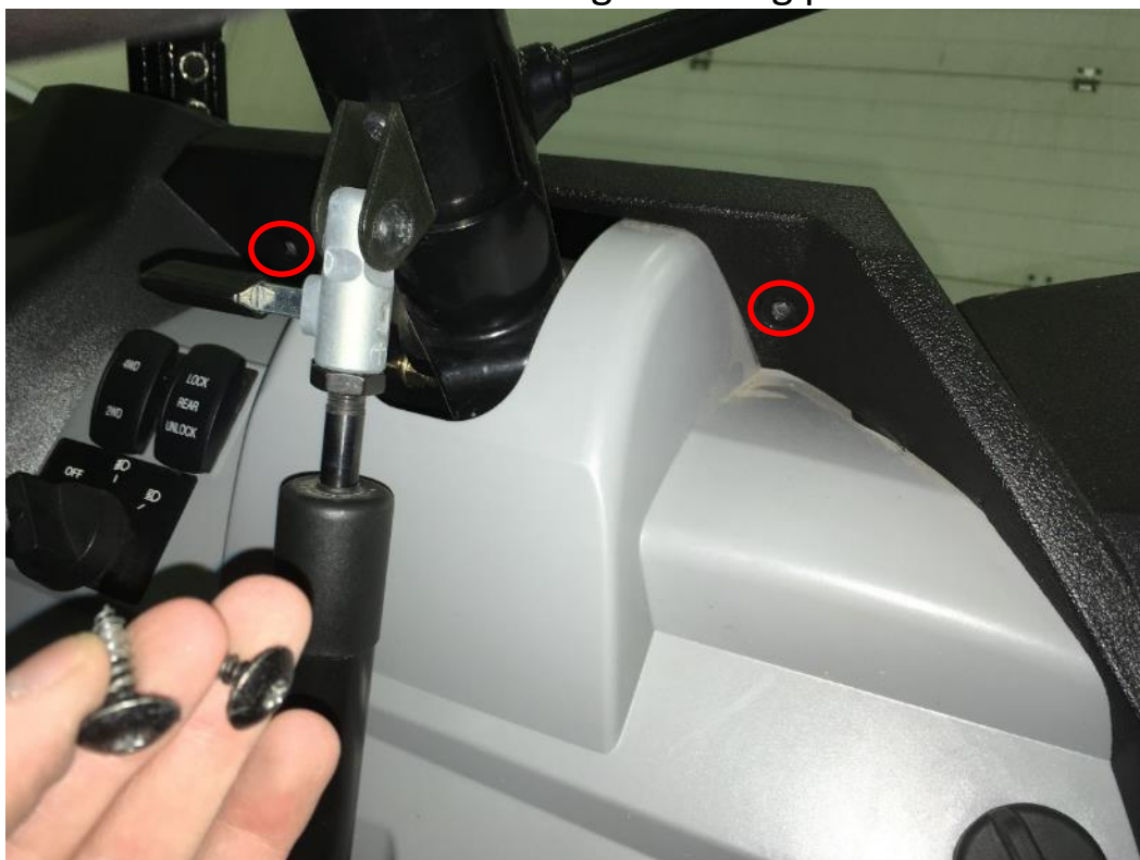
Detail view onto original fixing points.
