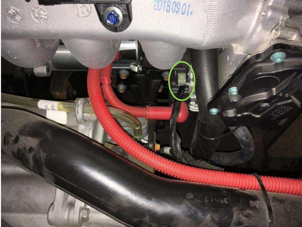
Take out the original connector and carefully uninstall the connector from the original harness.
