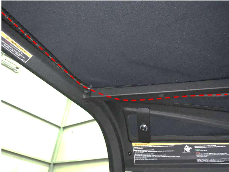
Connect the washer harness with the front wiper assembly.
