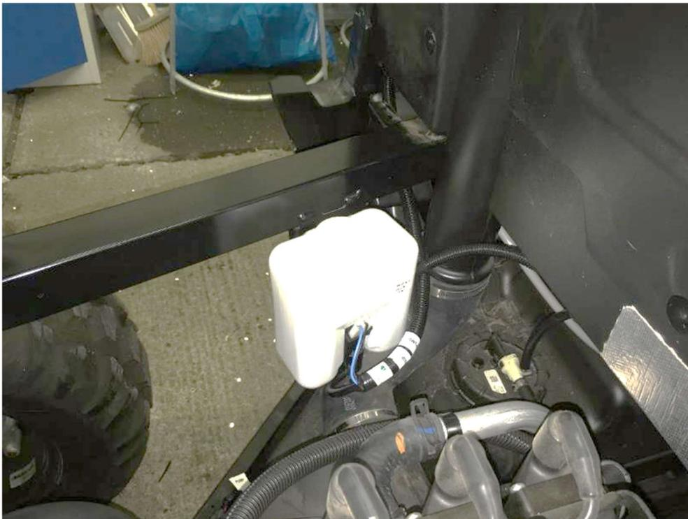
Connect the washer harness and washer hose with the washer tank.
