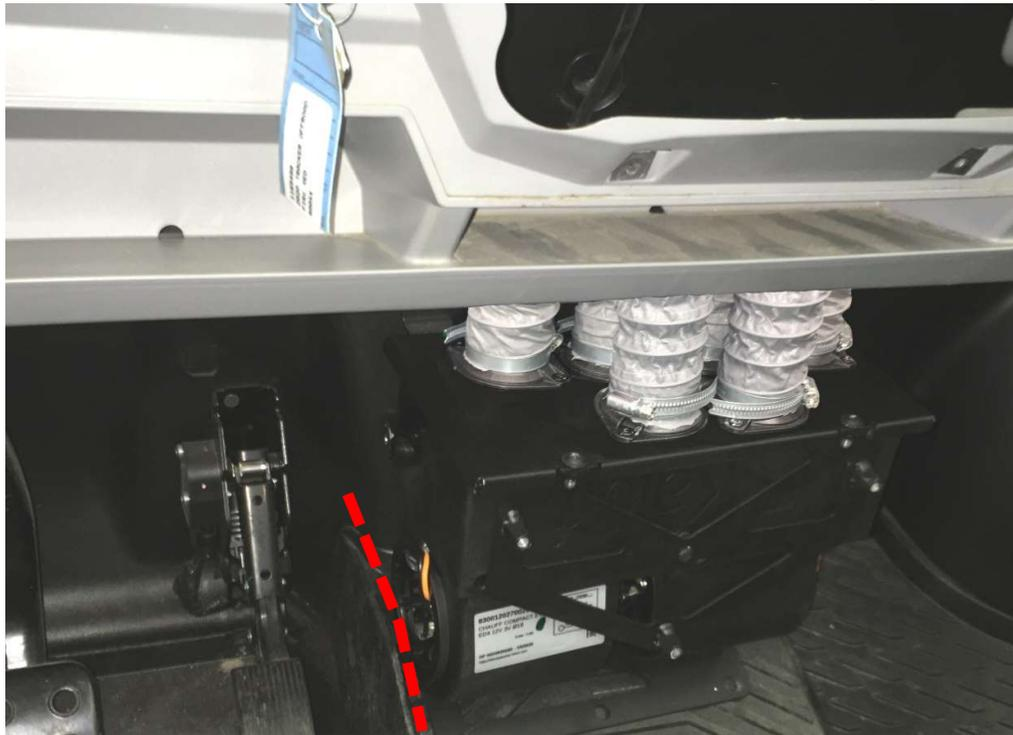
Make marks on the tunnel floor and front cover in accordance with the heater holder holes.
