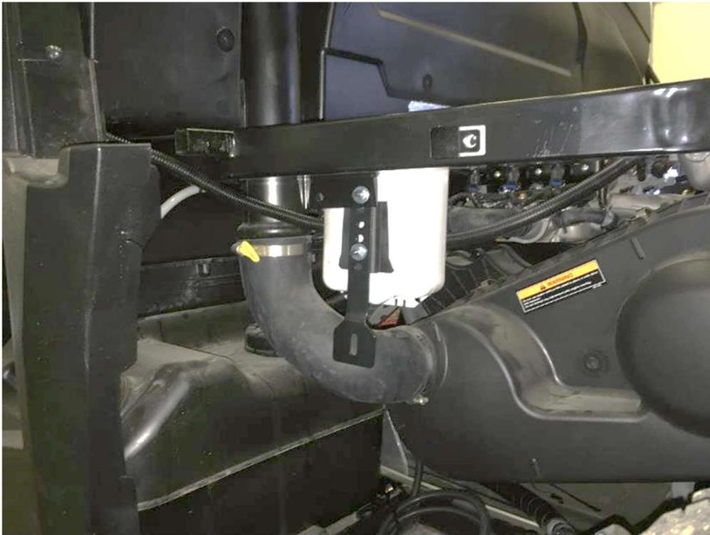
Place the washer tank onto the holder.
