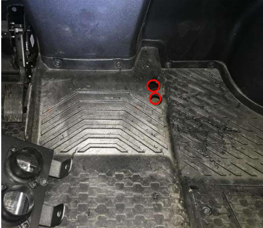
Drill hole  $\varnothing$ 20mm for heater harness.
