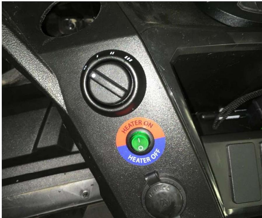
Connect the heater harness with the fan switch.
