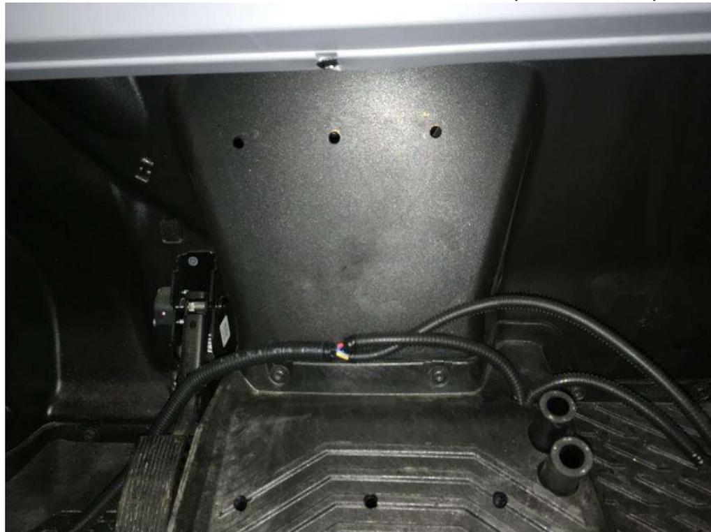
Drill holes  $\varnothing$  25mm for heater hoses.
