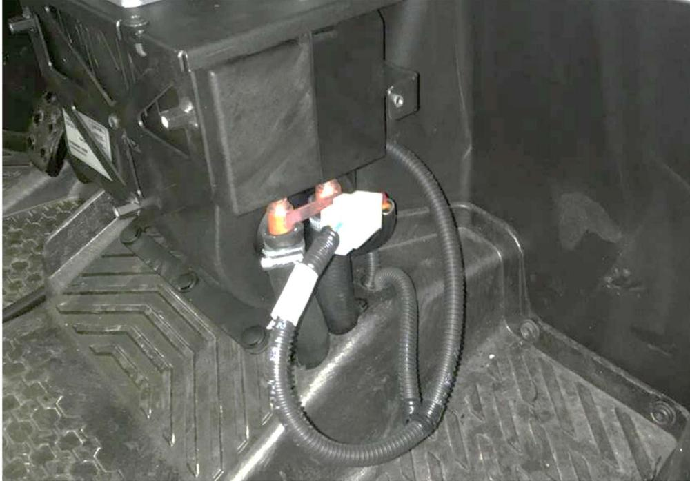
Connect the pump harness with the el. Valve.
