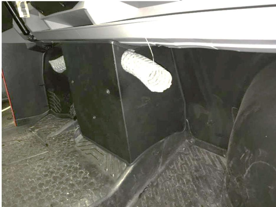
Install the air vents onto the hoses. Secure the vents with the hoses by included tightening straps. Push the air vents into the heater cover.
