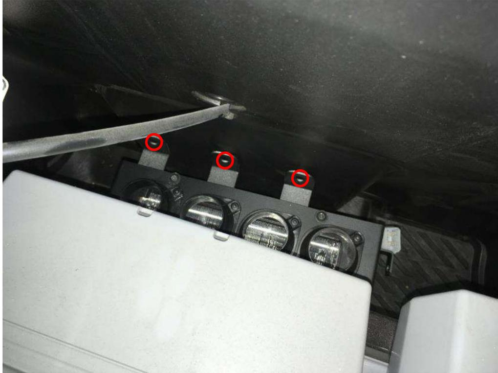
Drill 6 holes  $\varnothing$  8mm in marks centers from previous steps.
