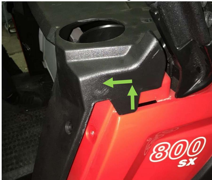
It is recommended to get the heater close to the floor tunnel edge, so the heater cover is in line with aforementioned edge.
