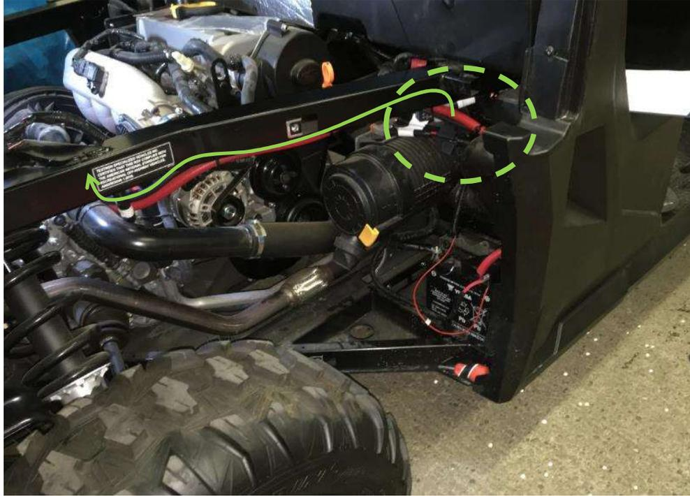
Run the ACC harness branch from the supply harness to the engine space.
