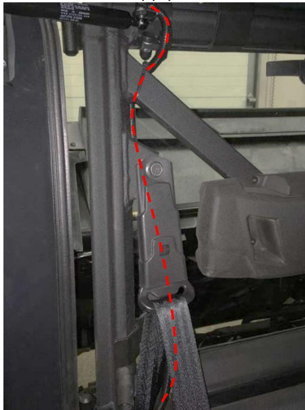
Run the wiper harness from the supply harness to the front wiper motor.
