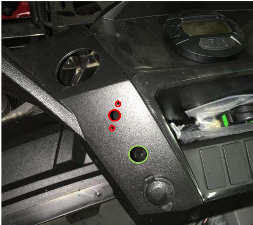
Install switches into the holes.
