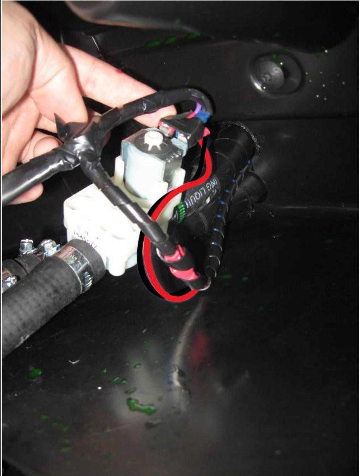
Connect the water pump harness onto the el. Valve.
