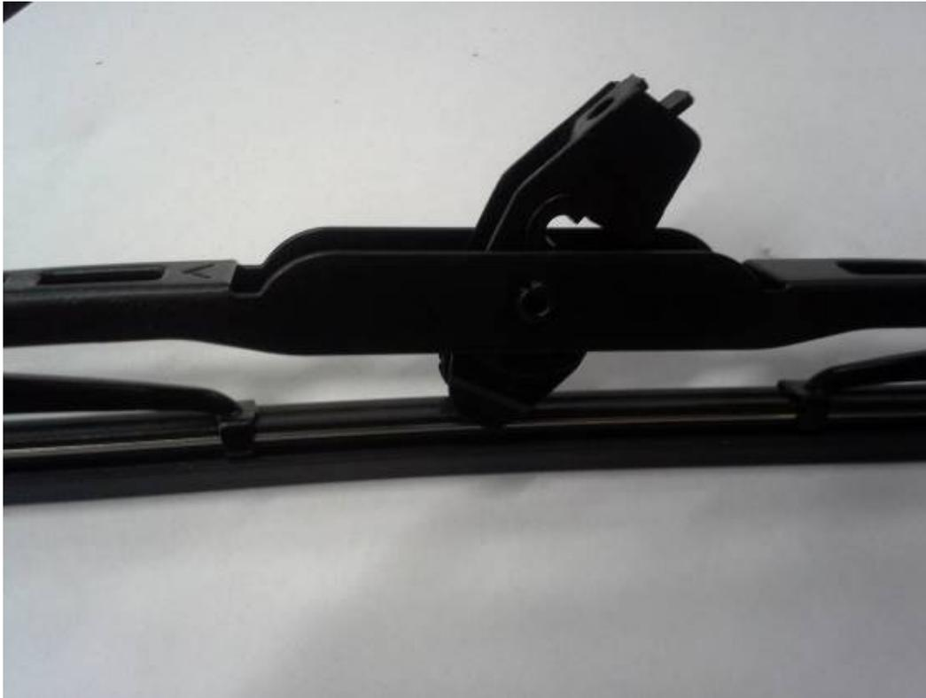
Insert the wiper arm hook onto the wiper latch plastic holder and press it into the correct position.
