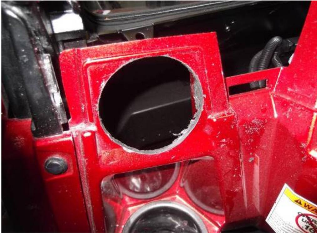
Cut the edge carefully from inner side. Repeat these steps on right dashboard side. Insert the air hose into the heater air tube and fix by included "AL" self glued tape.
