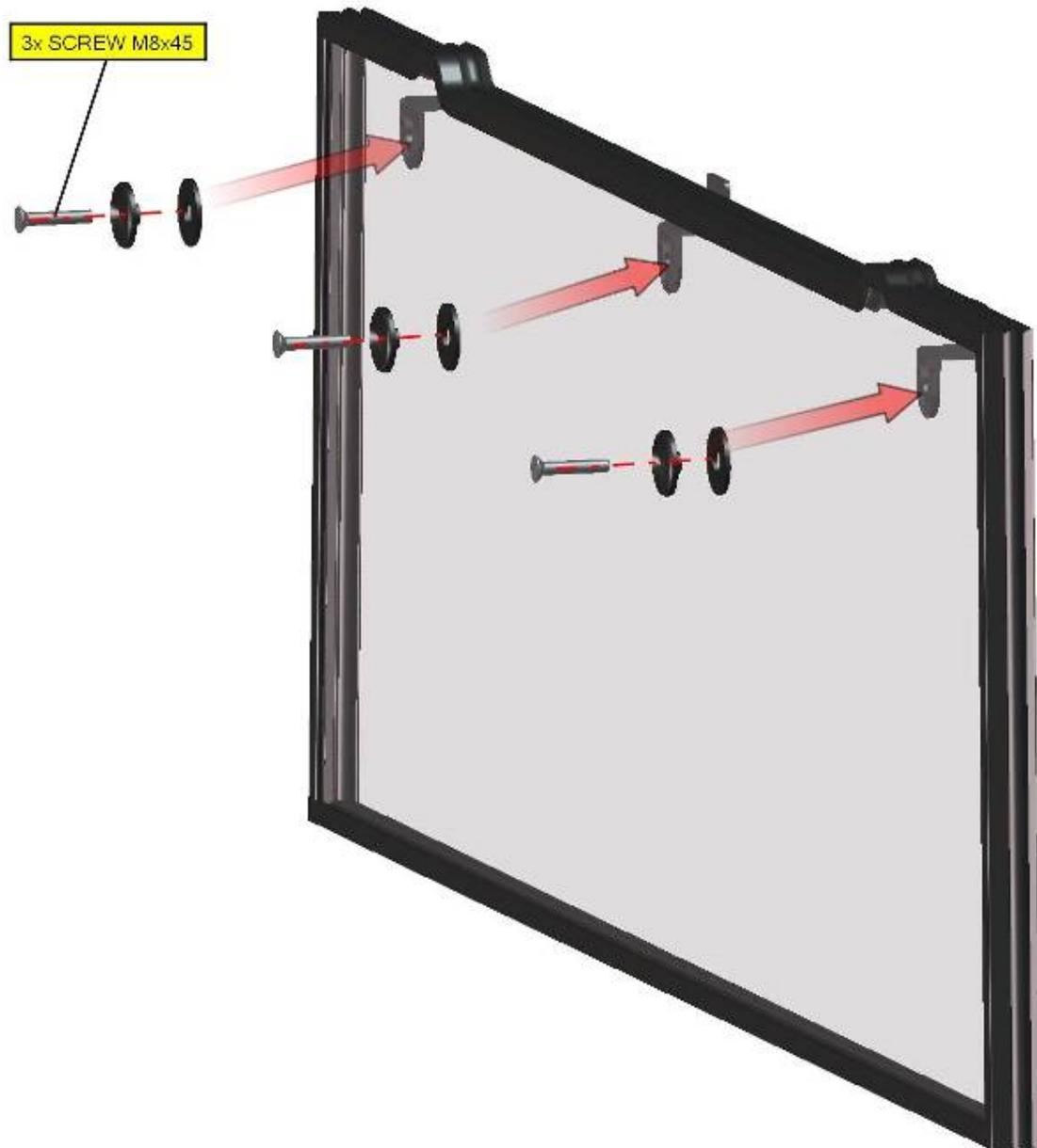
Fix the glass with the holders by screws and fast-lock handles and don't tighten these.
