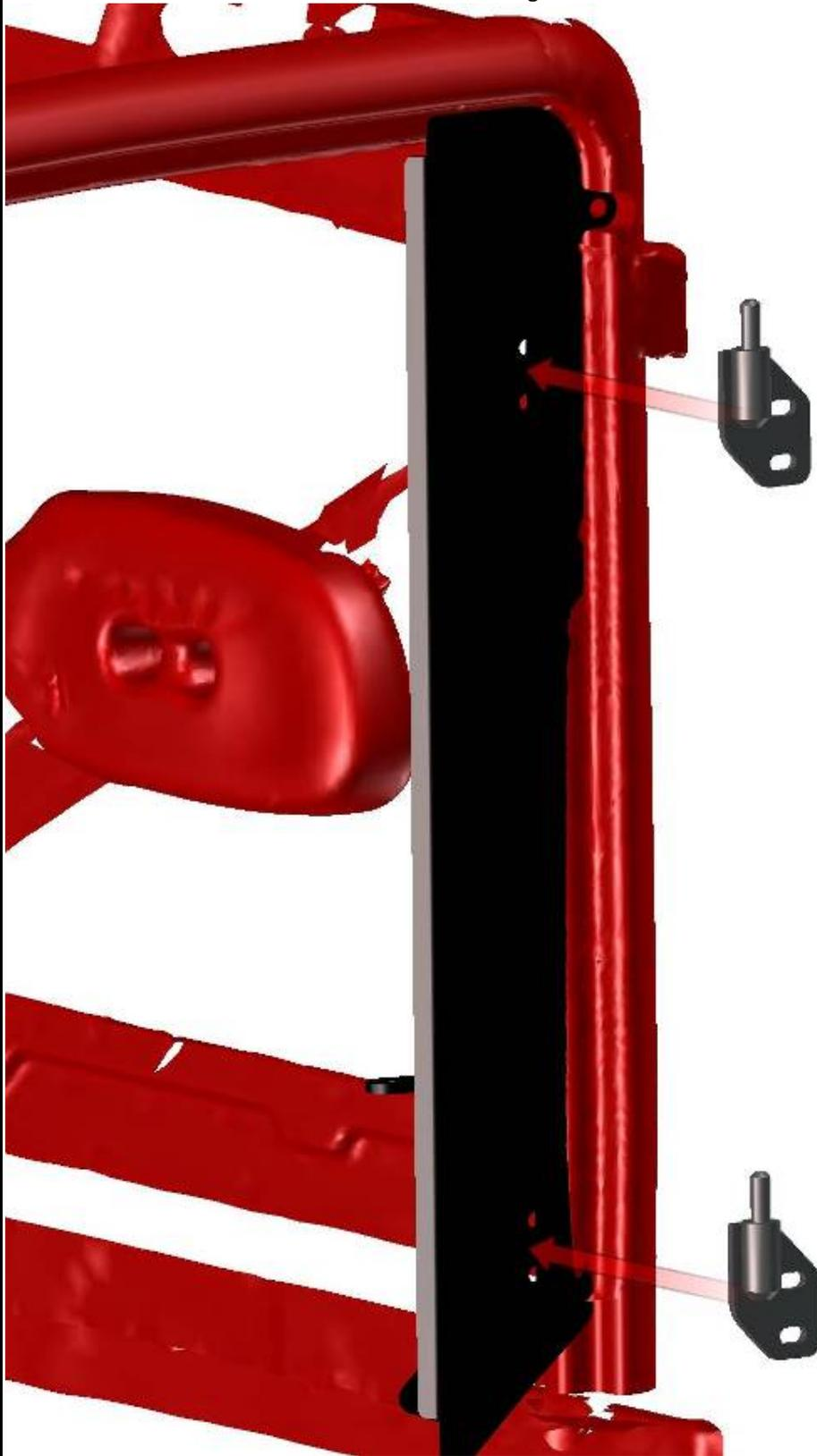
Fix the hinges with the door base and with the door base ledge by screws, washers, nuts and nut covers.
