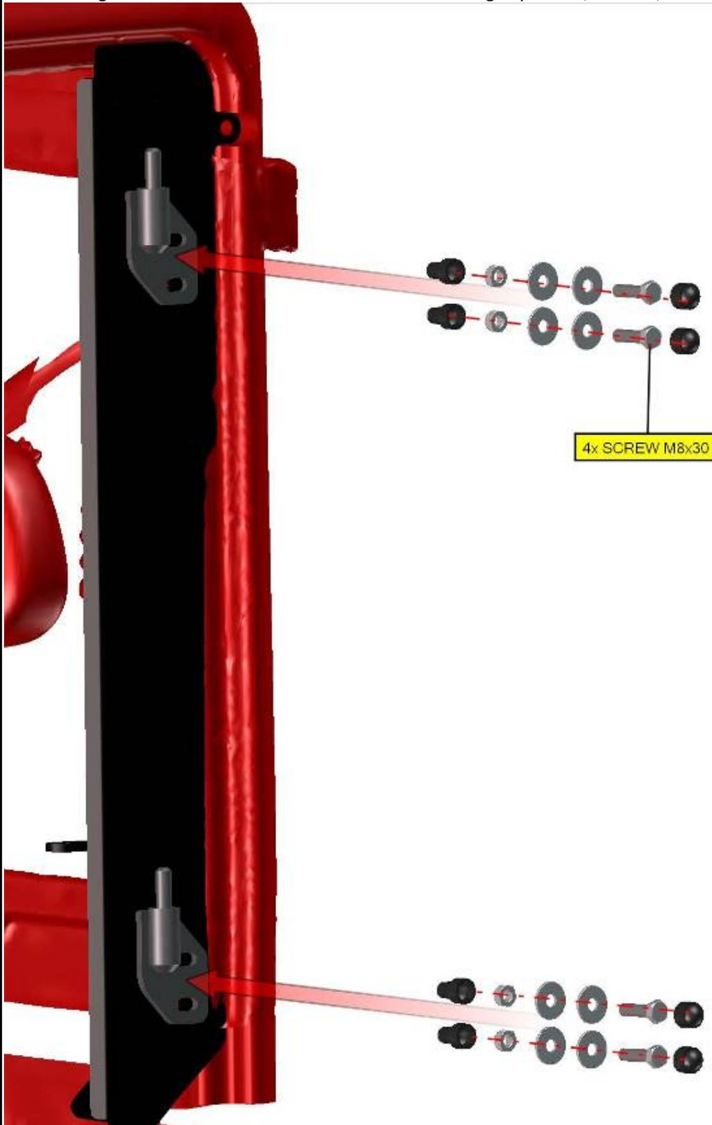
Place the door base holder onto the door base and onto the roller cage.
