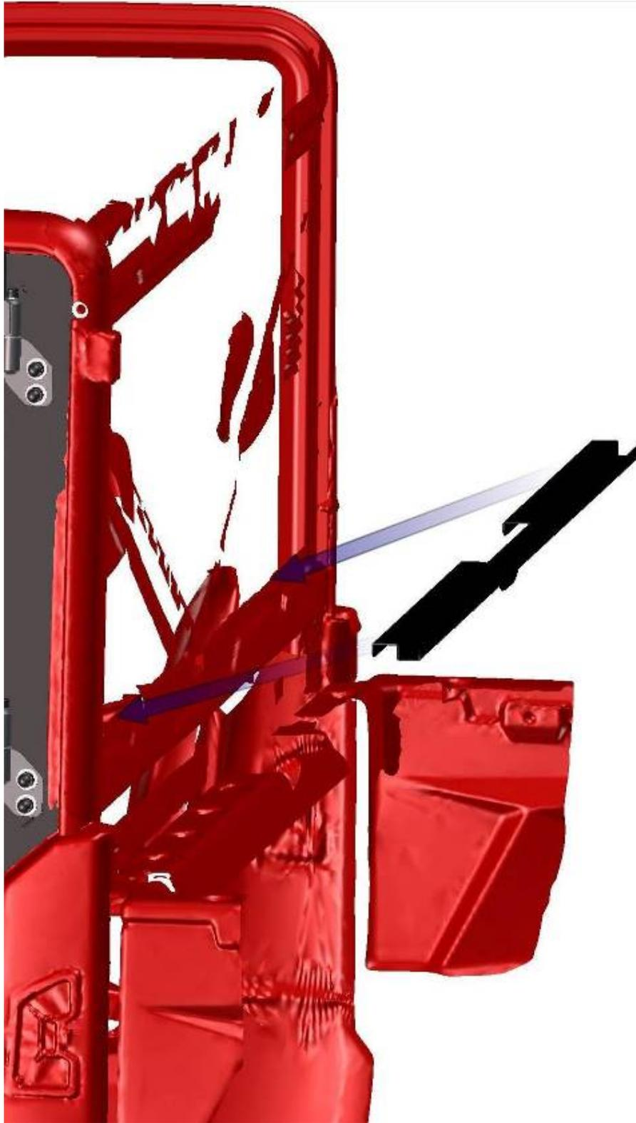
Place the rear glass holders onto the rear glass.
