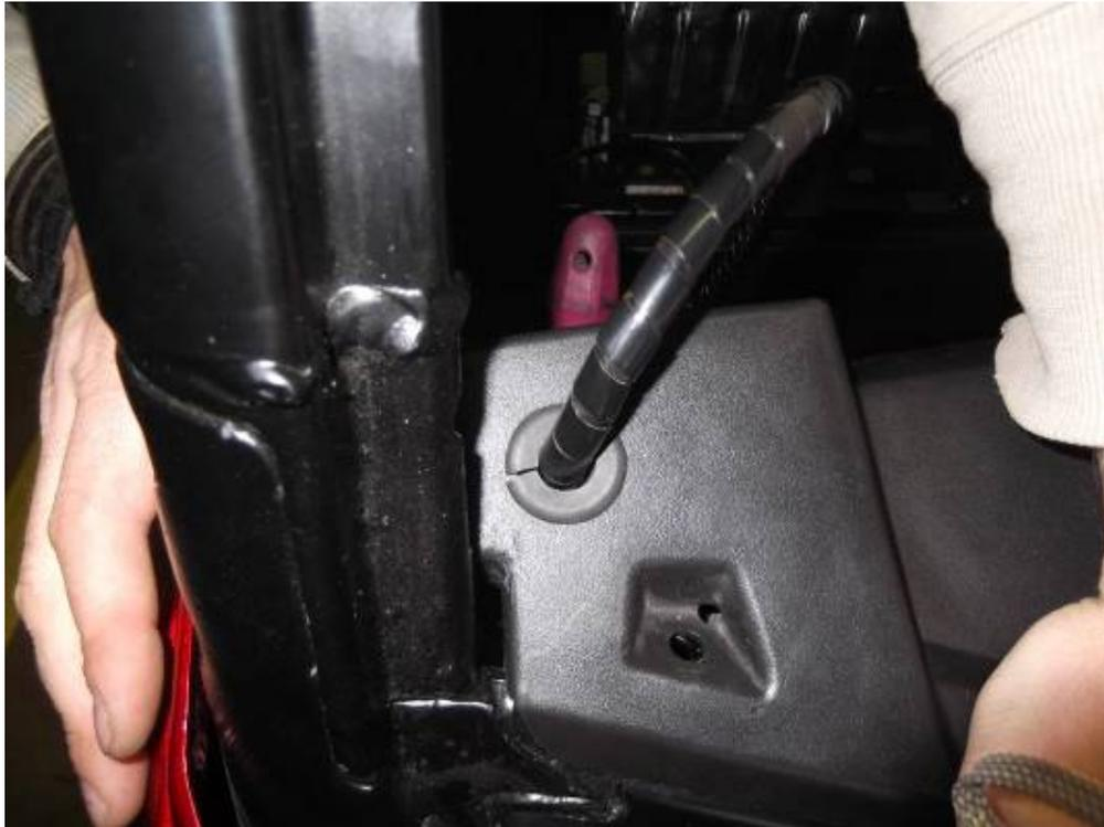
Connect the harness branch with the wiper motor connector.
