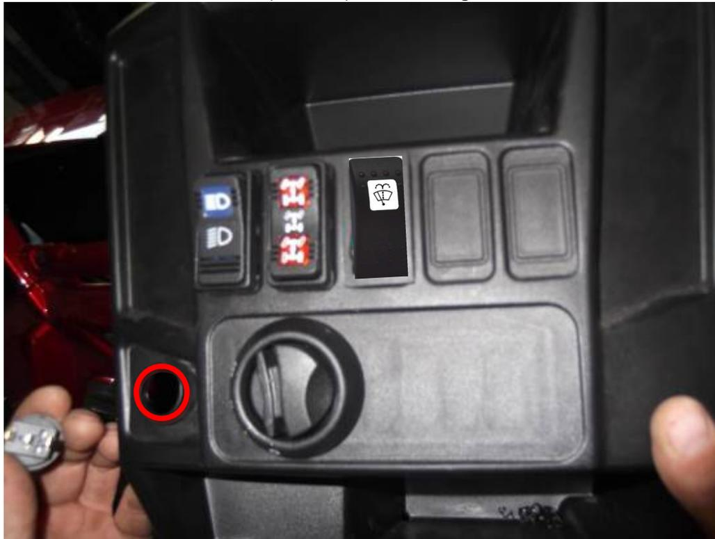
Pull the harness branch No.: 2 through the hole from previous page (bottom picture) and connect the branch with the switch. Detail of connection.
