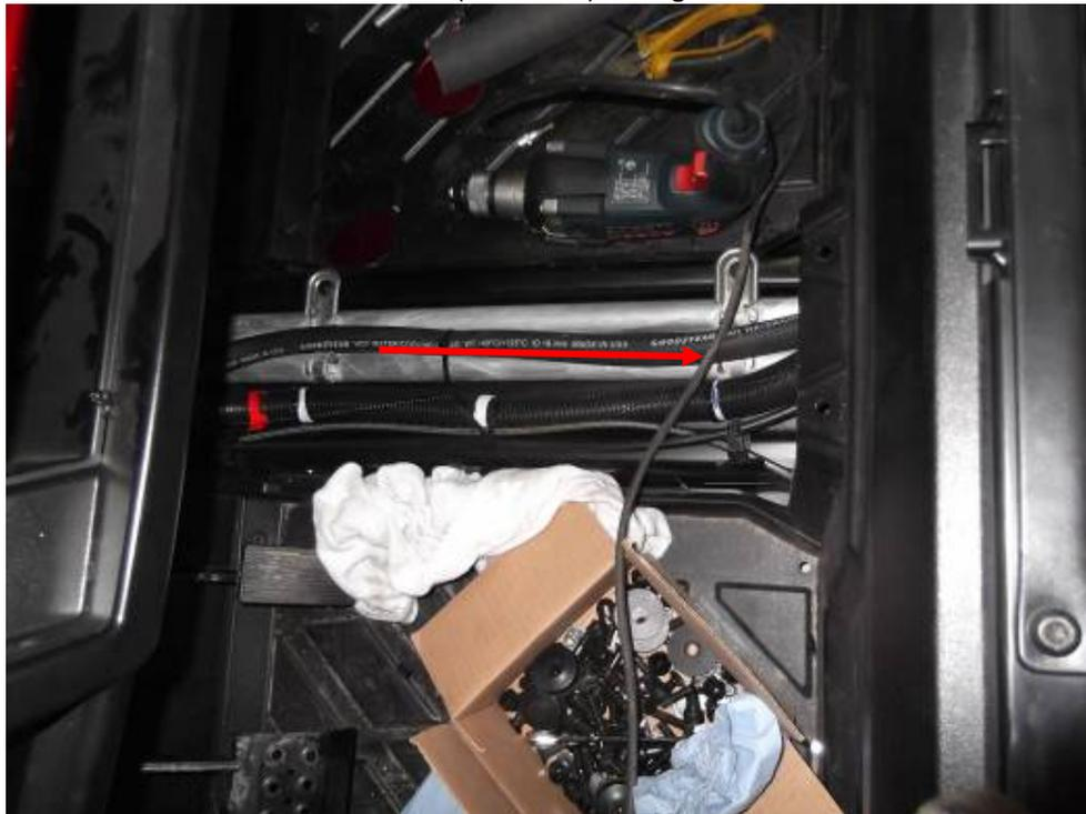
Cut the water hose (with red line) to correct length, be carefull to not cut that hose too short.
