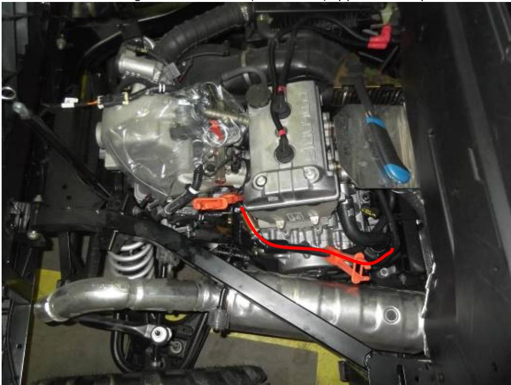
Cut the hose between pliers and insert tightening straps at loose ends. Install the small “Y” coupling into the original hose and into the heater hose (included). Tighten all (3) straps hard and lead the water hose from the engine to the central floor tunnel. It is necessary to keep the heater hose (red arrow) in direction of down and forward. **Side view.**
