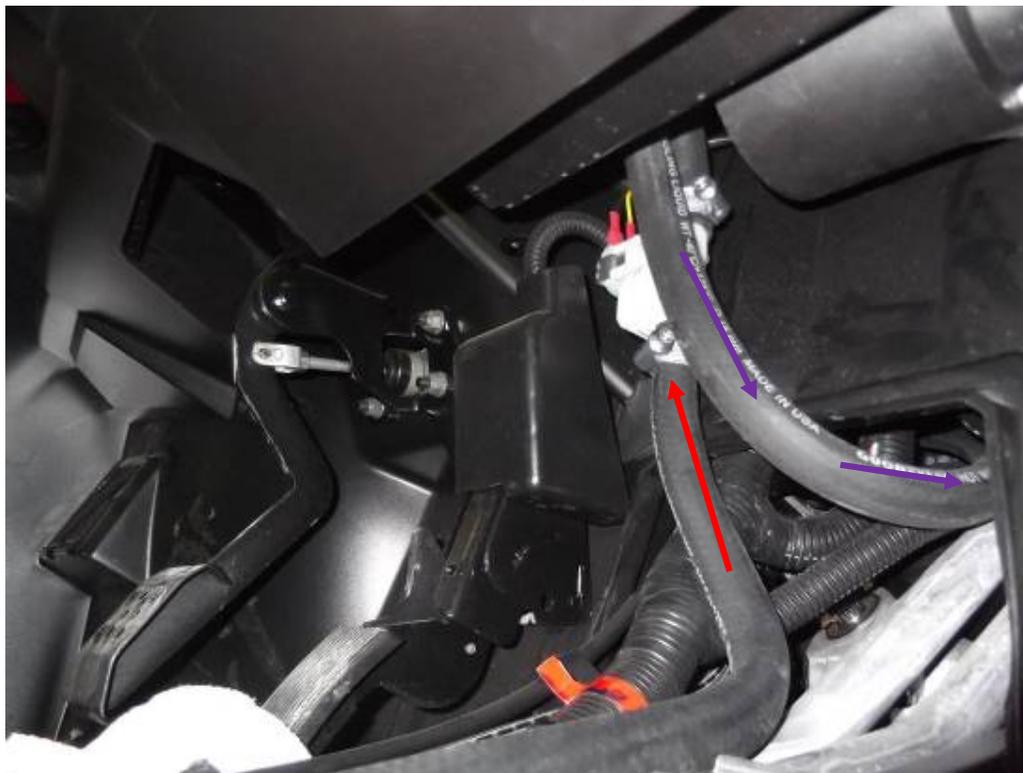
Secure vertical original hot water hose (with red line) near the left wheel by pliers or clamps from page No.: 12. Cut the vertical hose between the pliers and insert the tightening straps onto the hose.
