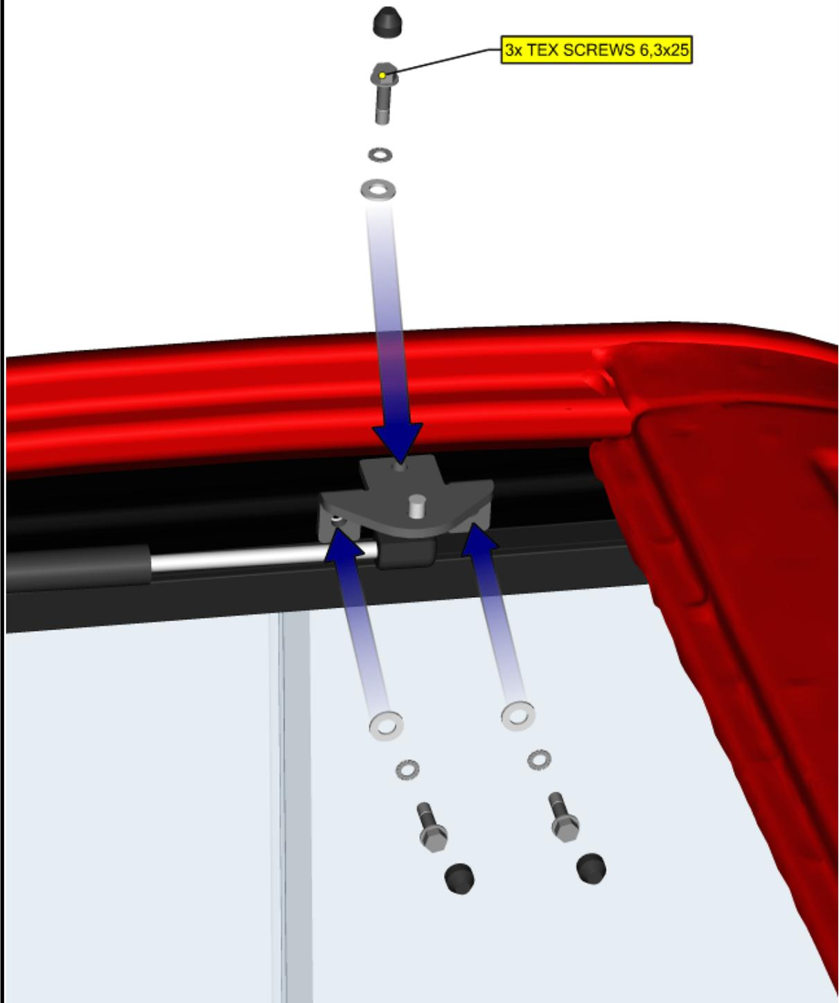
Fix the gas spring with the holder by nut, washer and nut cover.
