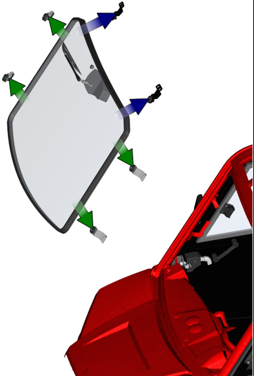
Place the front window onto the vehicle frame.
