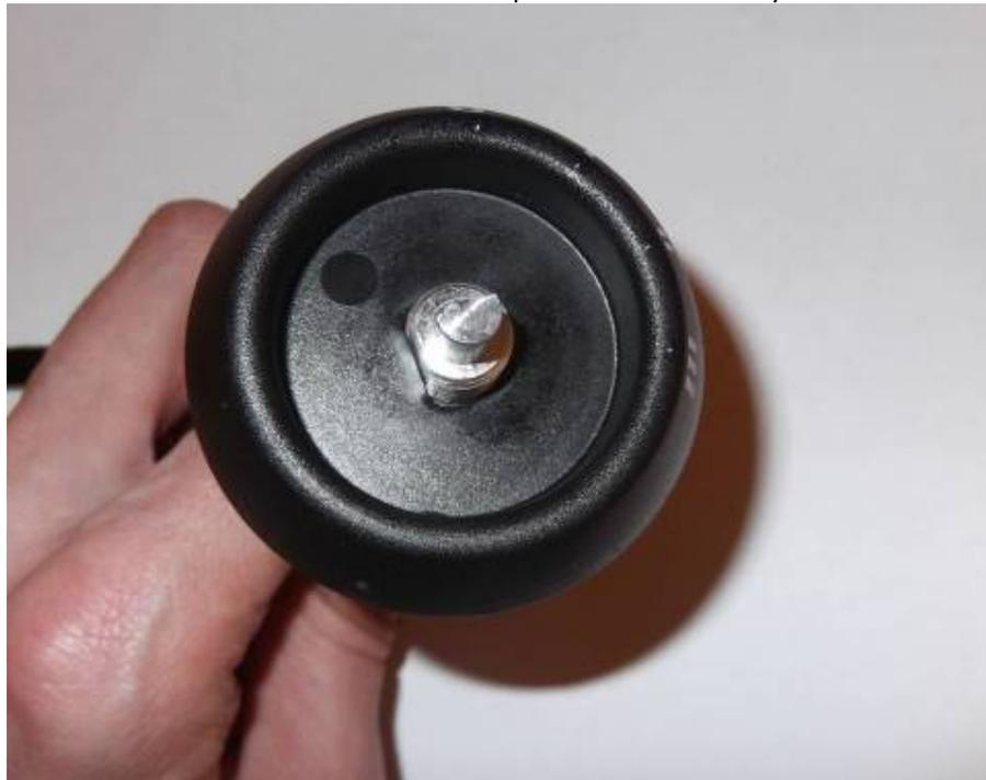
Fix the switch with the switch base to dashboard by nut.
