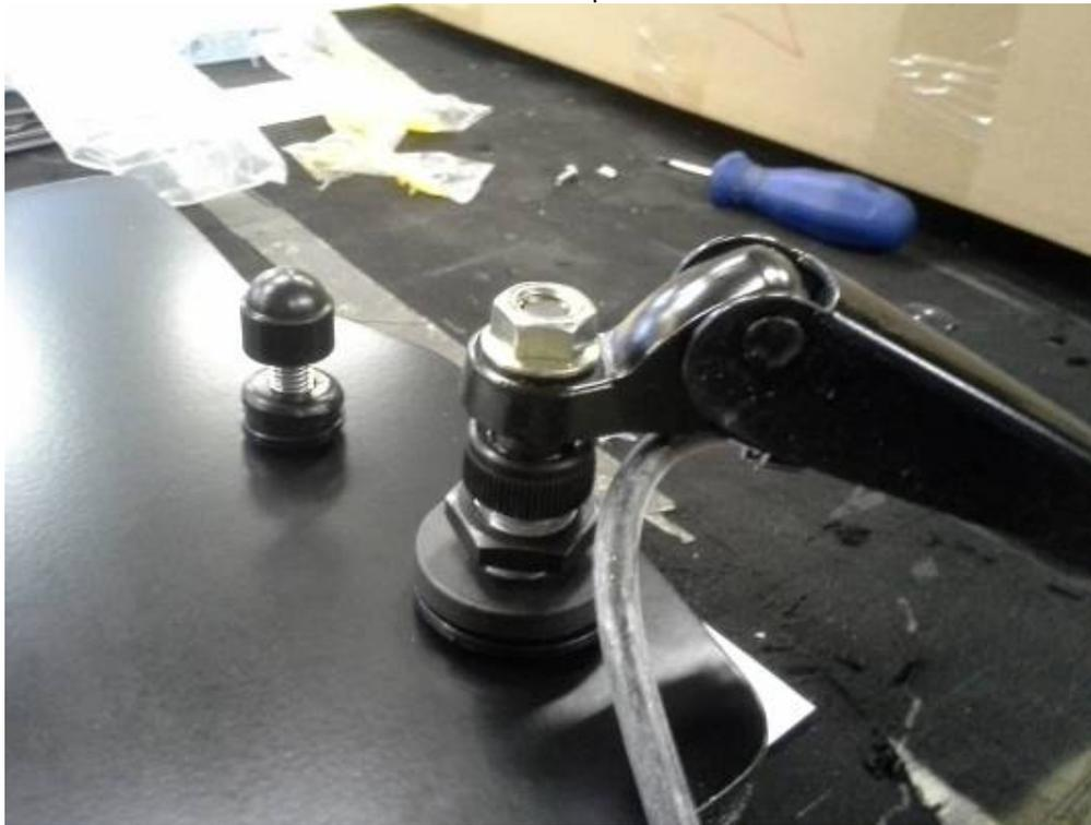
Fix the wiper arm with the wiper motor pin by included nut.
