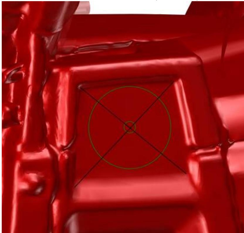
Cut the holes  $\varnothing 56\text{mm}$  (2,2 in) into the dashboard, use hole from previous step like pivot.
