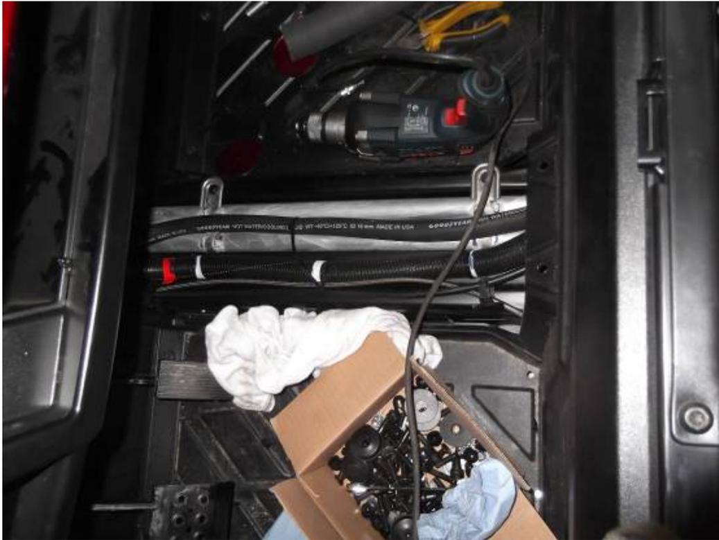
Secure original hot water hose (with red line) by pliers or clamps.
