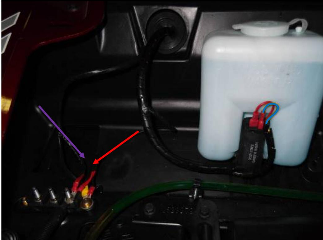
Connect the branches with the UTV' electroinstallation. Detail of connections.
