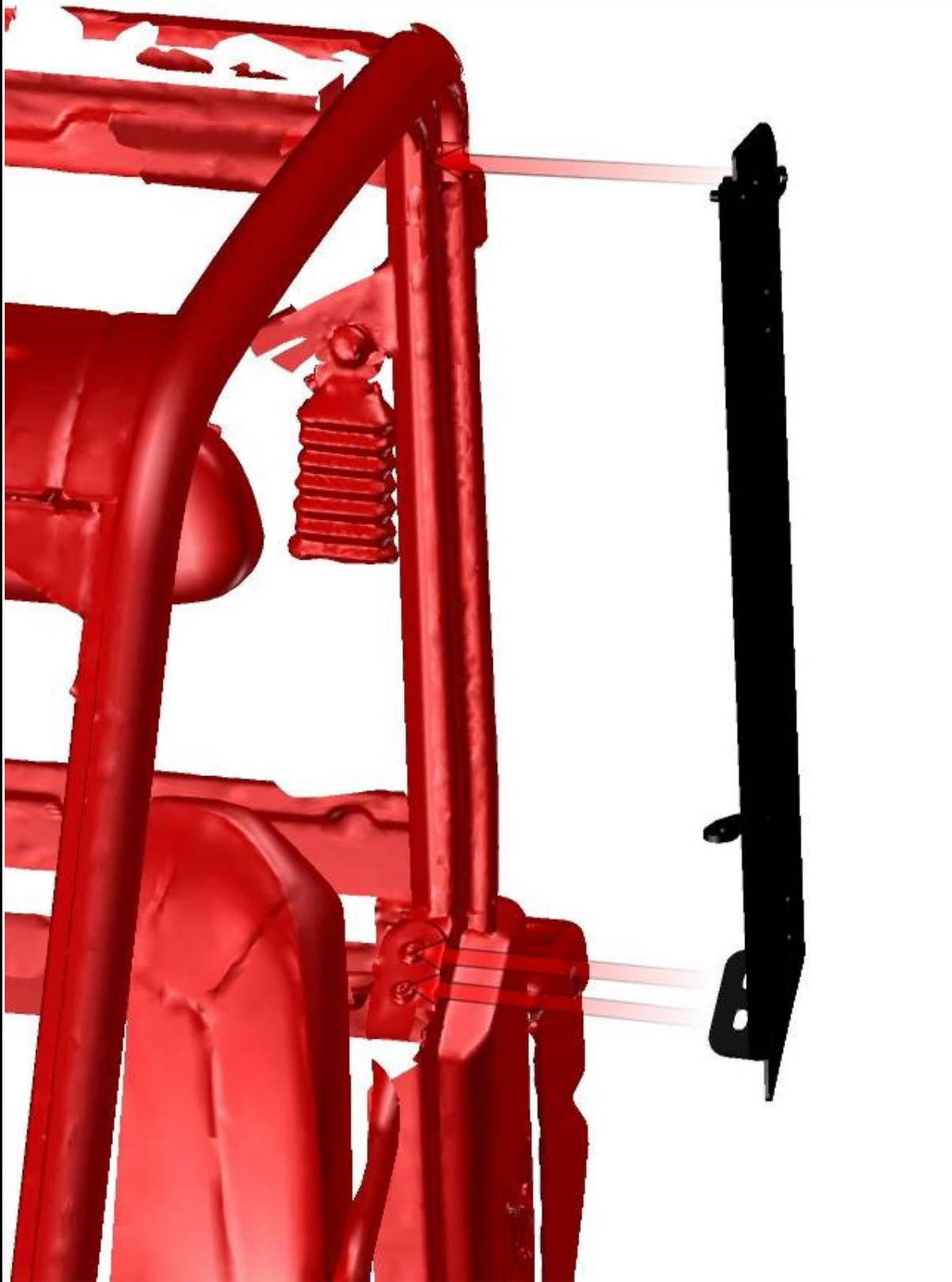
Fix the door base with the roller cage by original screws from page No.: 36.
