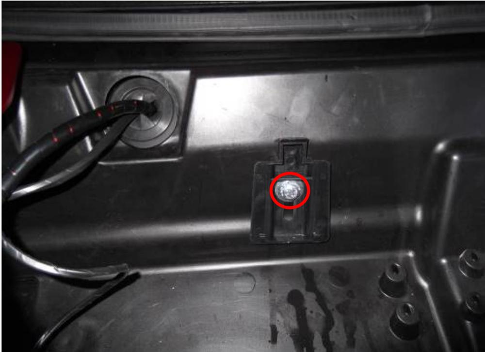
Connect the harness branch No.: 3 with washer motor and slide the washer tank onto the washer tank holder. Lead harness (red arrow) from the washer through the hole to the inner place in the dashboard.
