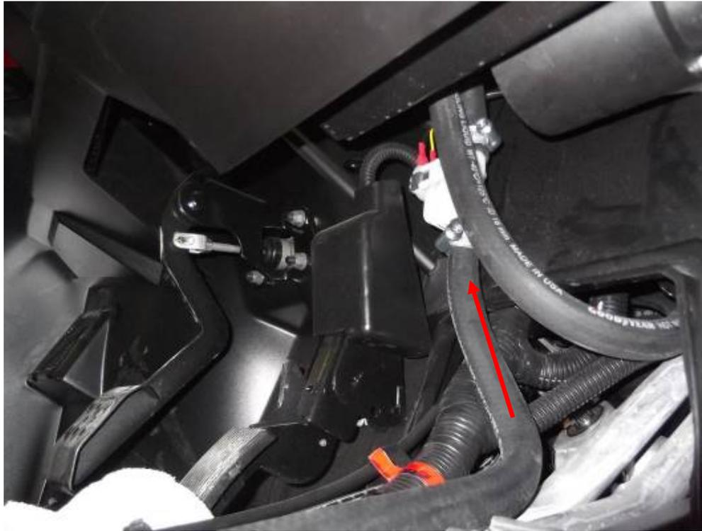
Install the short hose and remain of the hose to the heater tubes. Fix these hoses with the heater tubes by tightening straps and tighten these straps very hard. Insert the tightening strap onto the shorter hose and install electromagnet vent in same orientation like in picture. Tighten that strap very hard.
