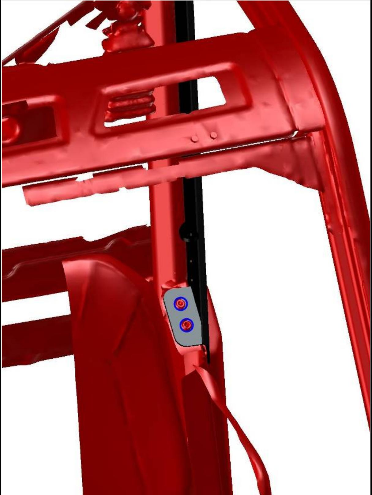
Fix the door base with the roller cage by original screw from page No.: 36.
