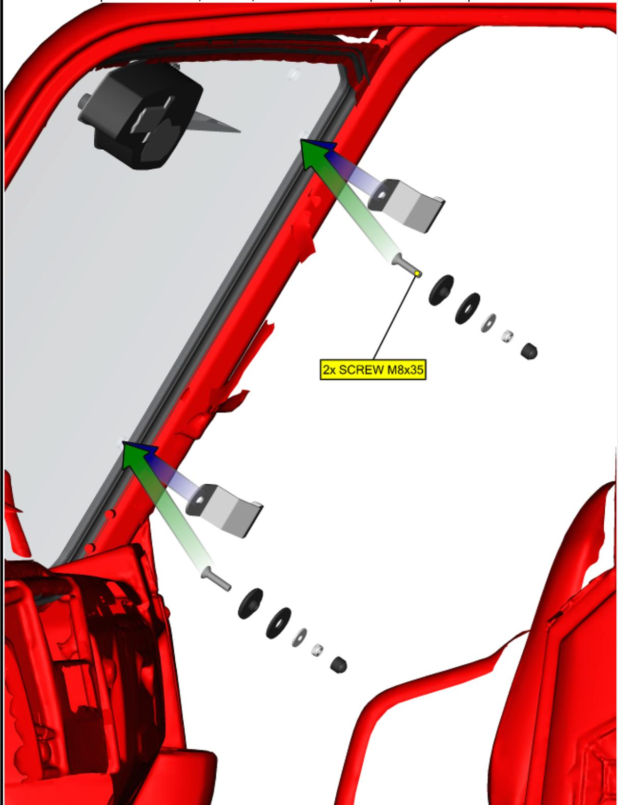
Place the front upper holder onto the window and onto the frame on both sides. Fix the holder with the window by included screw, washers, nut and covers on both sides. Adjust the window and the holders to the best position. Fix the holders with the frame by included screws, washers nuts and cover on both sides.
