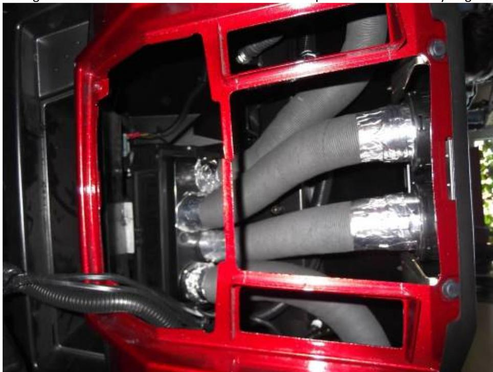
Stick the seal (black hide line) onto the UTV switch panel from inner side to upper edges and install panel back to position.
