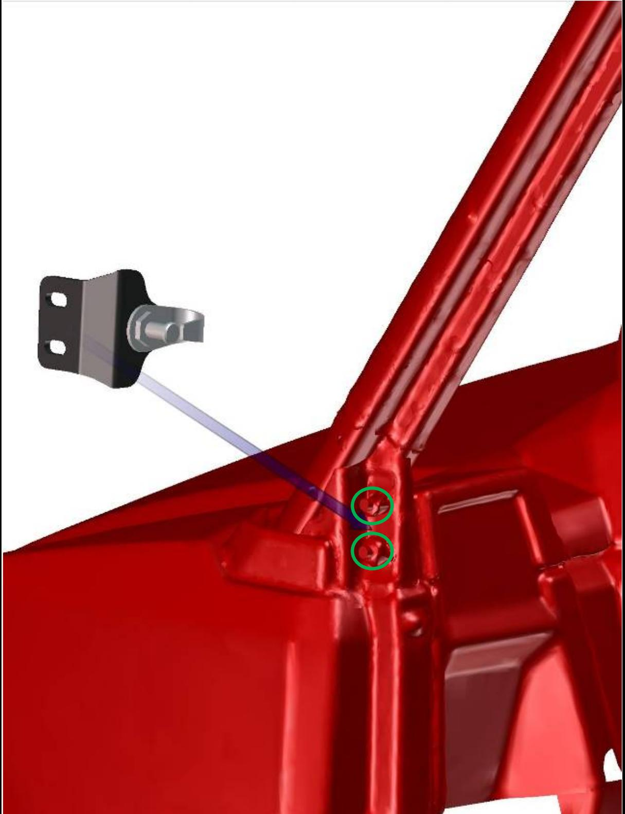
Fix the door stop holder with the roller cage by screws and washers.
