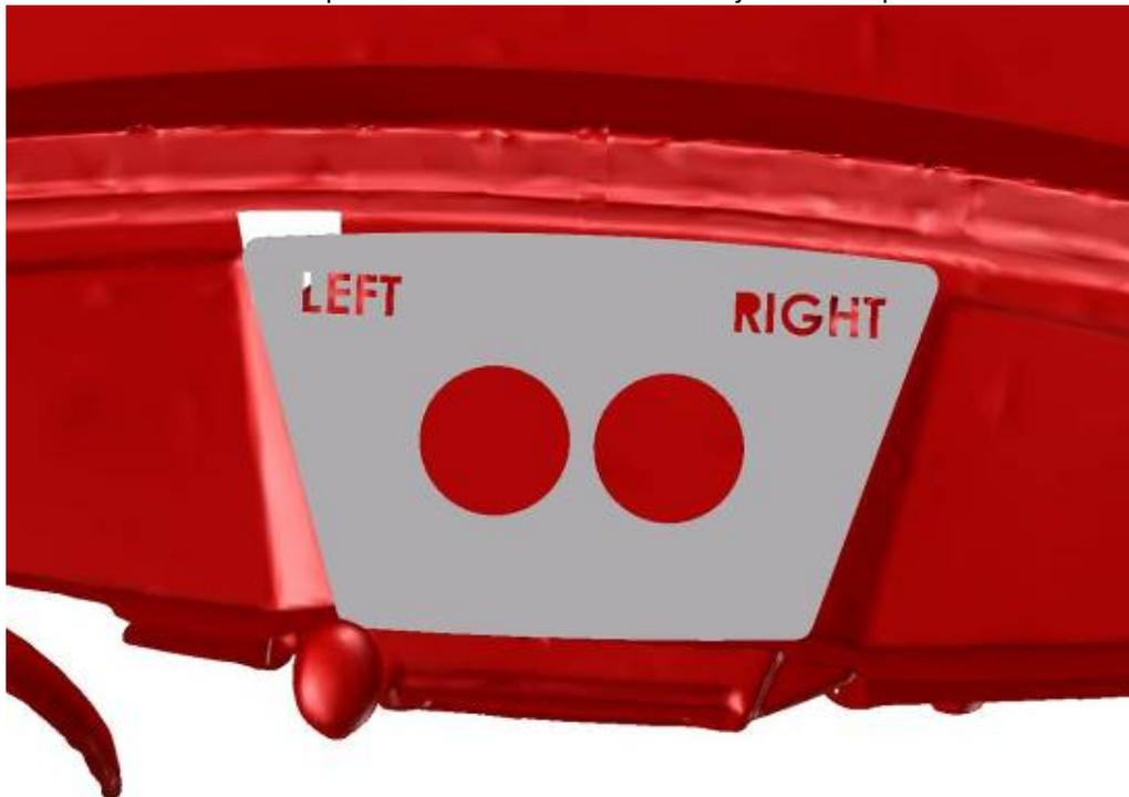
Make marks in accordance with the template and and cut the holes  $\varnothing 76\text{mm}$  (3 in) into the mark's centers.
