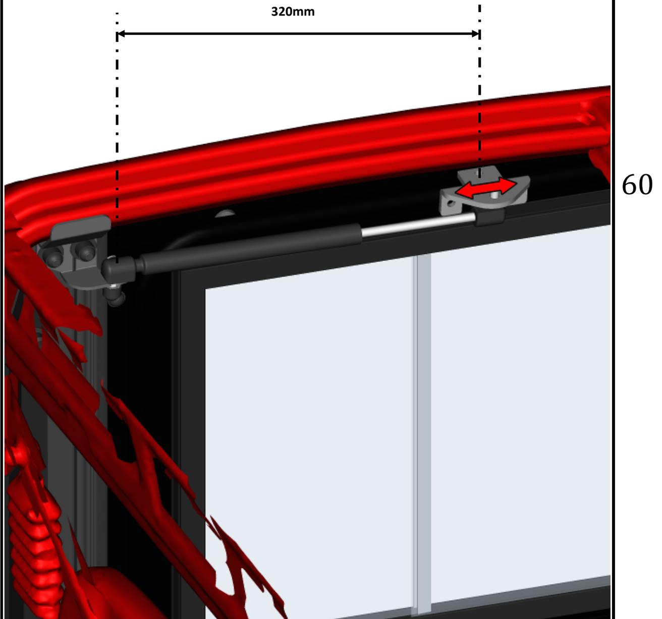
Fix the gas spring holder with the door frame by TEX screws, washers and TEX covers.
