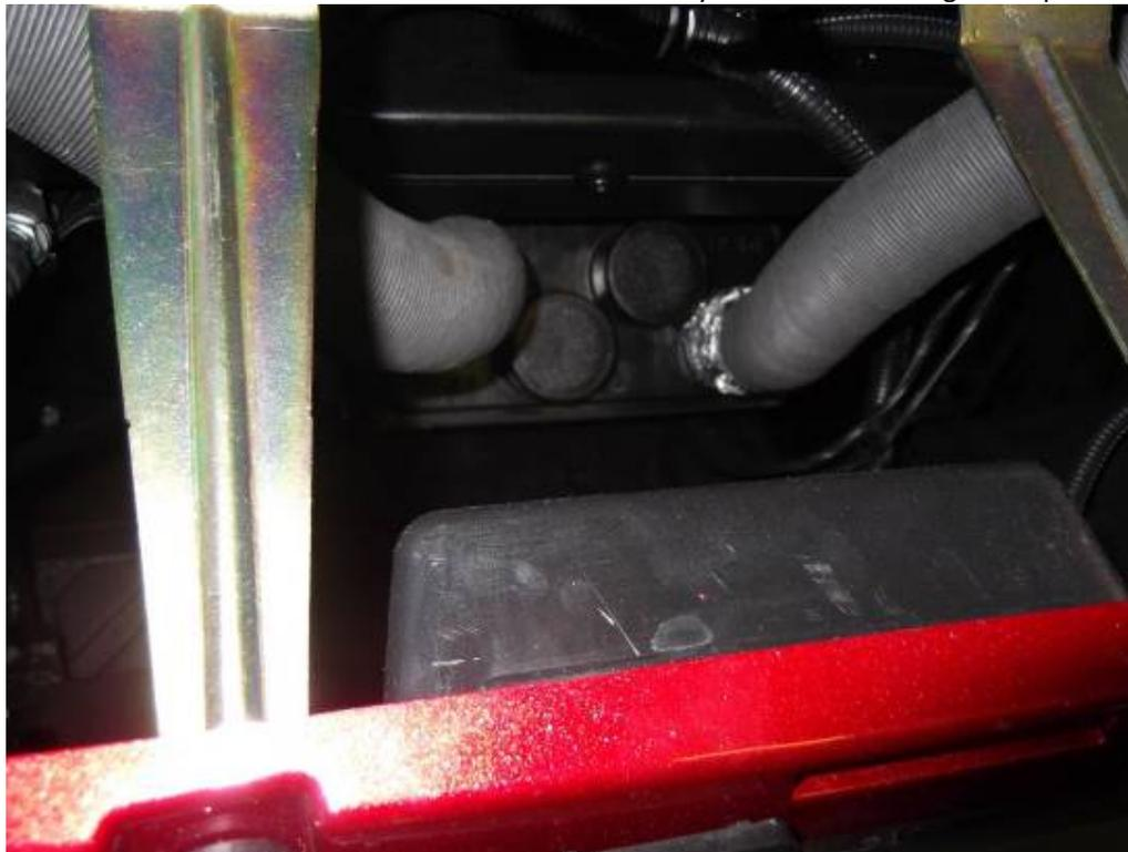
Lead air hoses to the roller cage. Insert air vent smaller into the hole. Insert tightening strap onto the air hose and insert the air hose onto the air vent smaller. Tighten strap hard.
