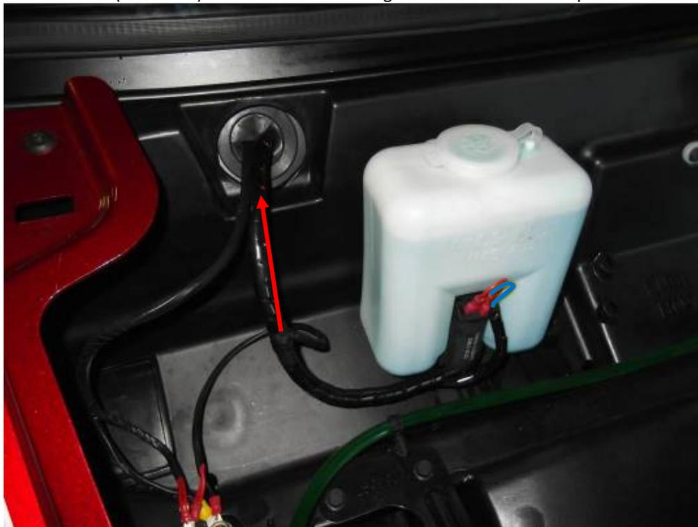
Lead the harness branch No.: 1 (red arrow) to the right front roller cage.
