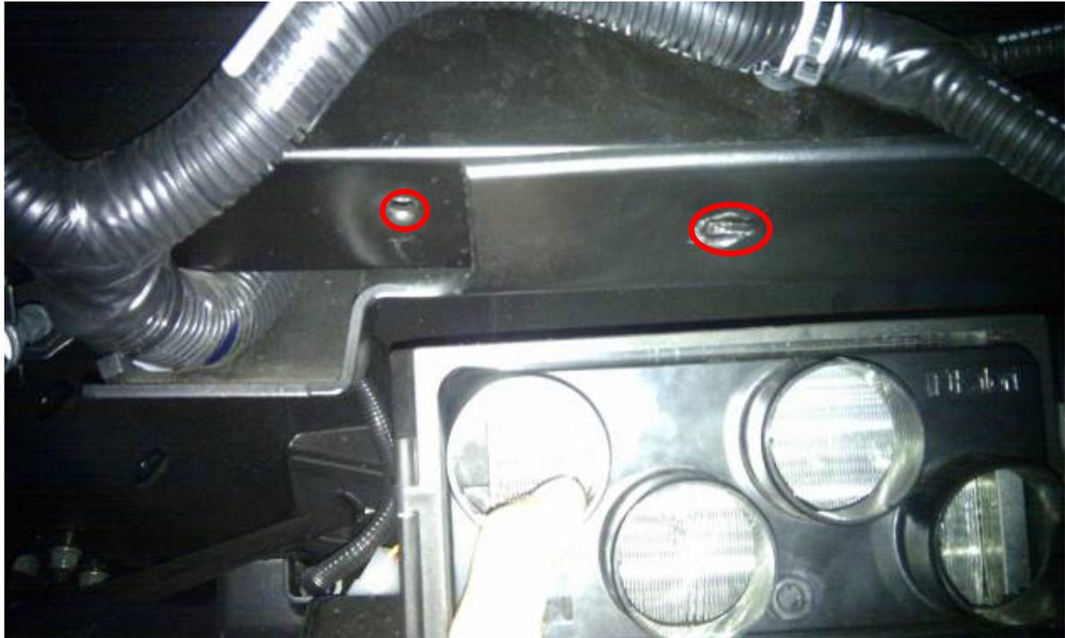
Connect harness branch No.: 3 with the heater connector. Detail view.
