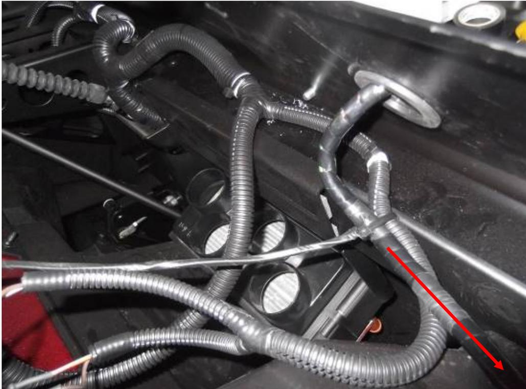
Drill hole (red circle)  $\varnothing$  21mm (0,83in) into the unmounted dashboard cover near the right roller cage and stretch the harness branch through the hole.
