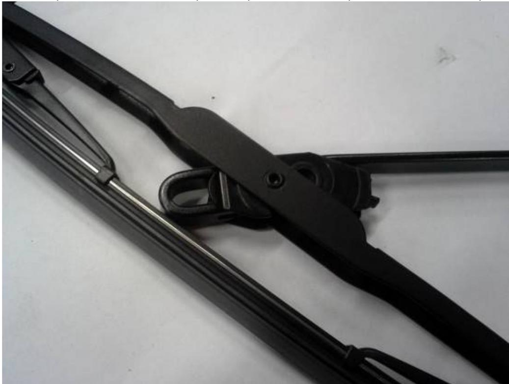
View onto installed wiper arm hook.
