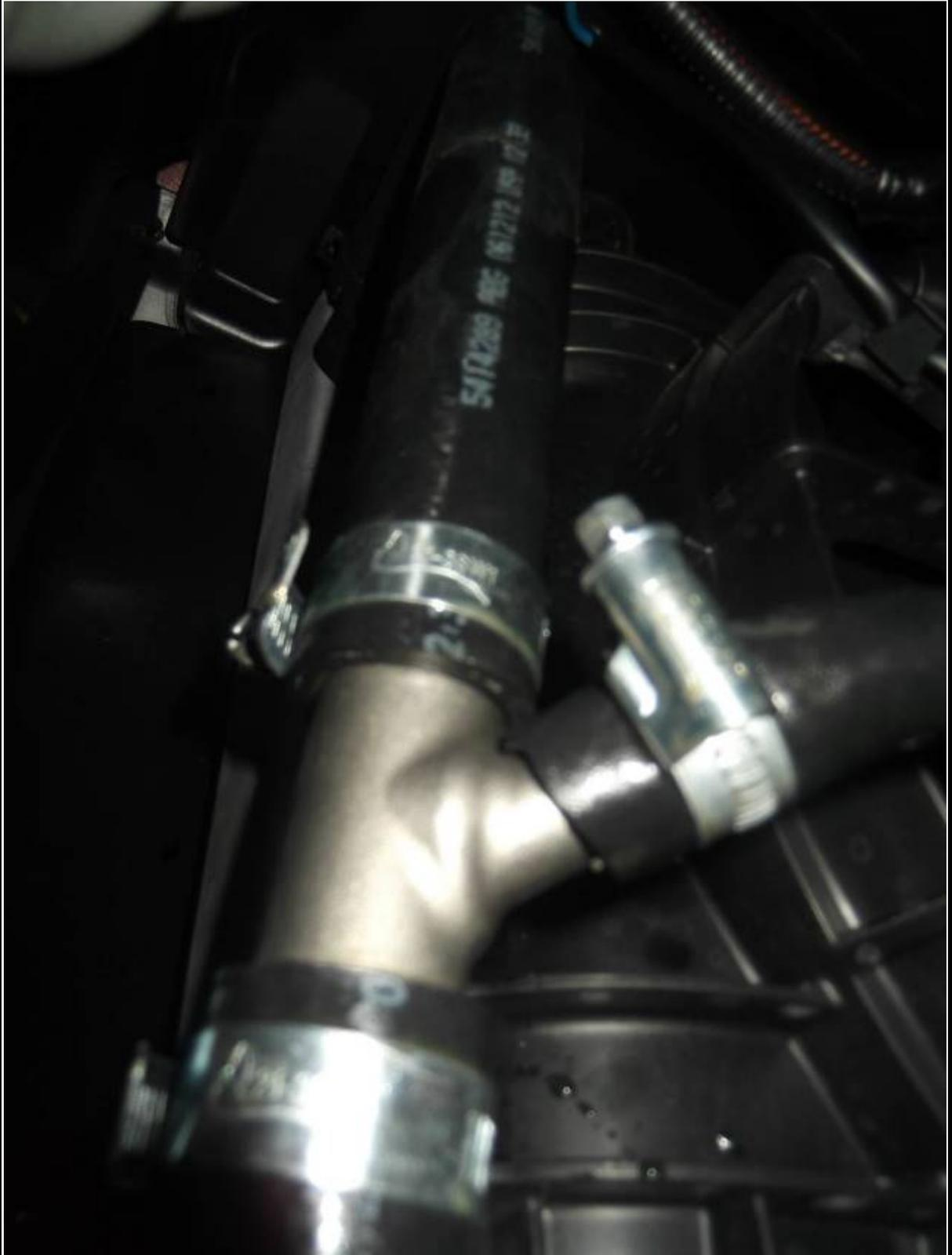
Cut the heater hose near "Y" coupling from previous page and insert the tightening straps. Install the air vent valve into the hose and fix these by straps. Tighten straps very hard.
