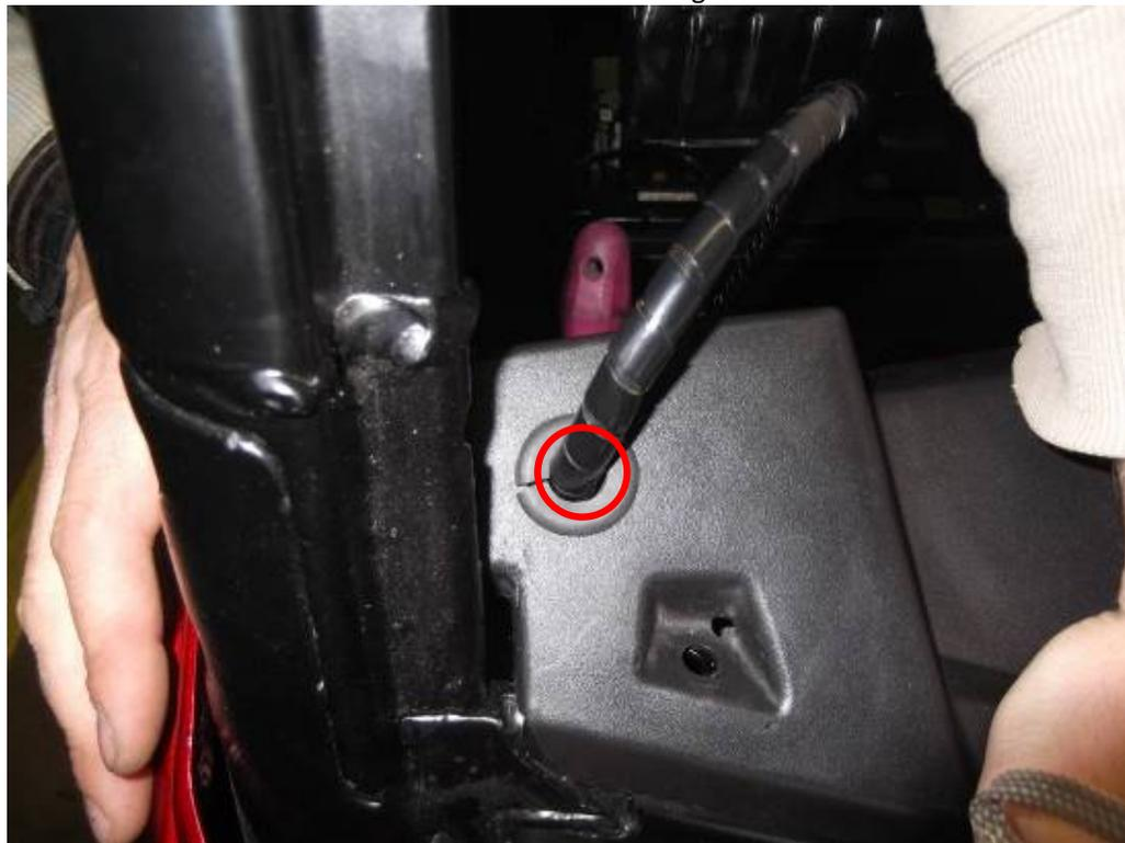
Uninstall the central panel from the dashboard and lead the harness branch.: 2 from the harness to the central panel.
