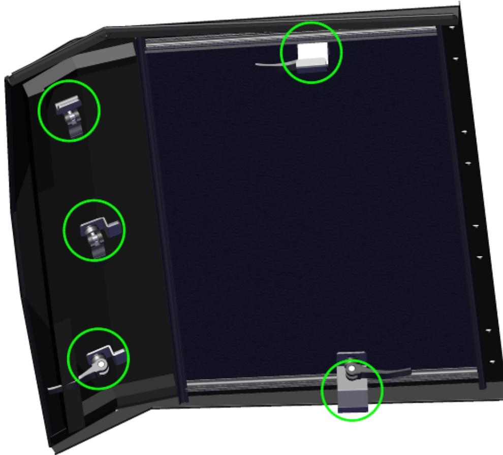
Place the front roof onto the rear roof and onto the UTV roller cage.
