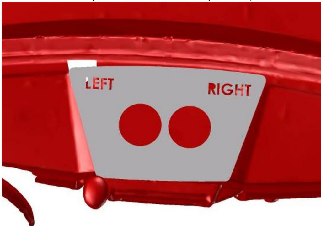
Make marks in accordance with the template and cut the holes  $\varnothing 76\text{mm}$  (3 in) into the mark's centers.
