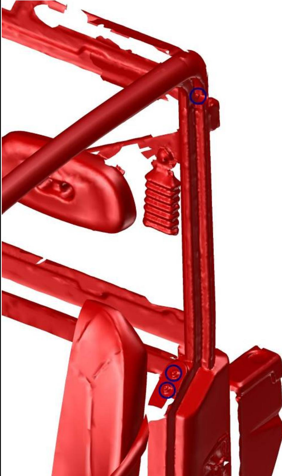
Place the left door base onto the roller cage and adjust that onto the best position.
