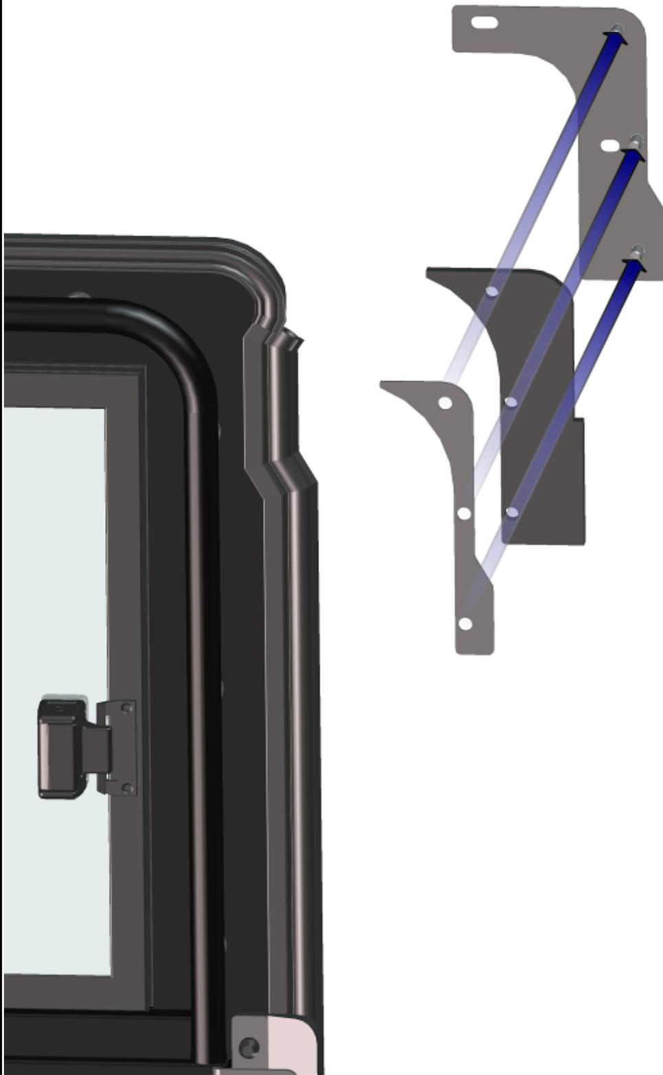
Fix the ledge and the EPDM onto the welded corner by nuts, washers and covers.
