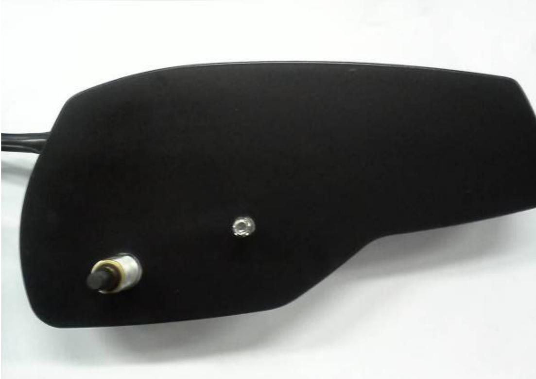
Place the washer onto the wiper longer pin.
