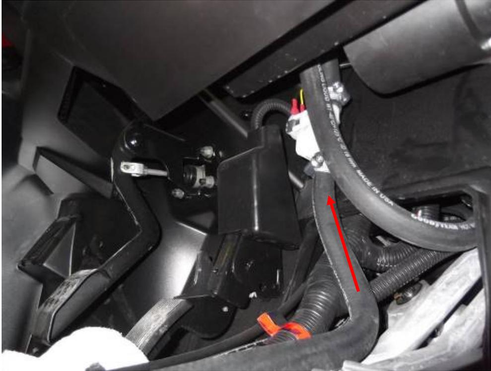
Install the short hose and remain of the hose to the heater tubes. Fix these hoses with the heater tubes by tightening straps and tighten these straps very hard. Insert the tightening strap onto the shorter hose and install electromagetic valve **in same orientation like in picture**. Tighten that strap very hard.
