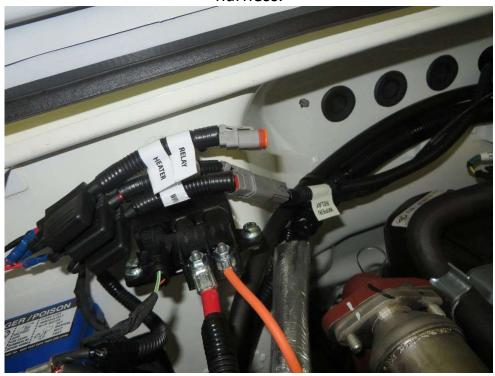
Run the washer harness to the washer tank. Connect the harnes with the washer tank.
