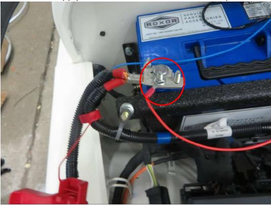
Connect supply harness BLACK WIRE with the battery 12V-.
