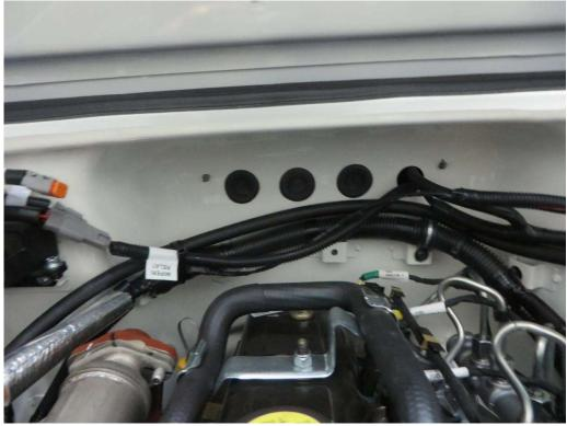
Place the wiper harness and washer harness onto the engine space.
