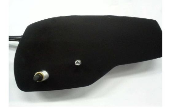
Place the washer onto the wiper longer pin.
