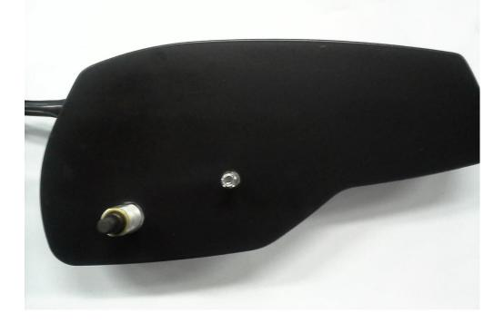
Place the washer onto the wiper longer pin.
