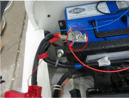
Connect supply harness BLACK WIRE with the battery 12V-.
