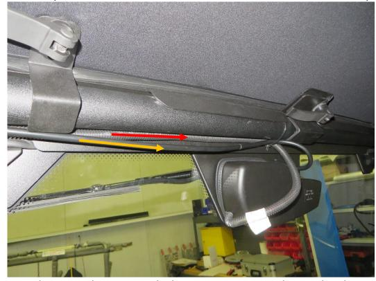
Connect the wiper harness with the wiper. Connect the washer hose with the washer jet.
