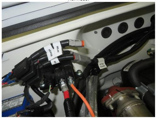
Run the washer harness to the washer tank. Connect the harnes with the washer tank.
