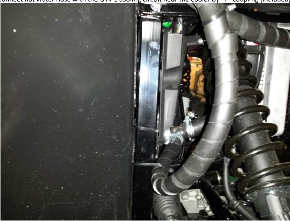
Lead the second hot water hose under the UTV floor to the engine.
