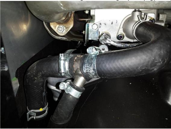
Connect the heater to the hot water hoses and to the heater harness and place the heater onto the heater holder and fix by included nuts, washers and covers on both sides.
