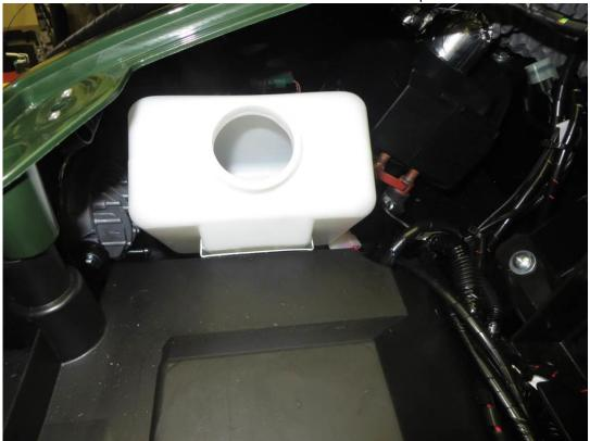
Lead the wiper harness branch with the washer tube alongside the right roller cage ledge.
