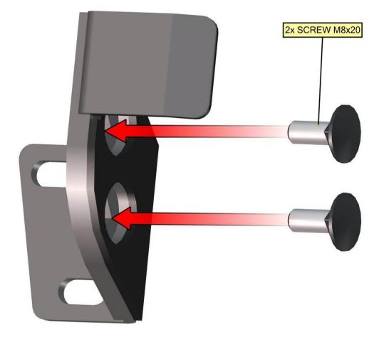
Place the front bottom ledge holder with the screws onto the front bottom ledge and fix by included screws, washers, nuts and covers on both sides. 2x SCREW M8x20
