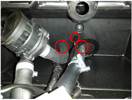
Install the hot water pump onto the hot water hose(red circle). Take extra care to the correct orientation. Connect the hot water pump to the pump harness.
