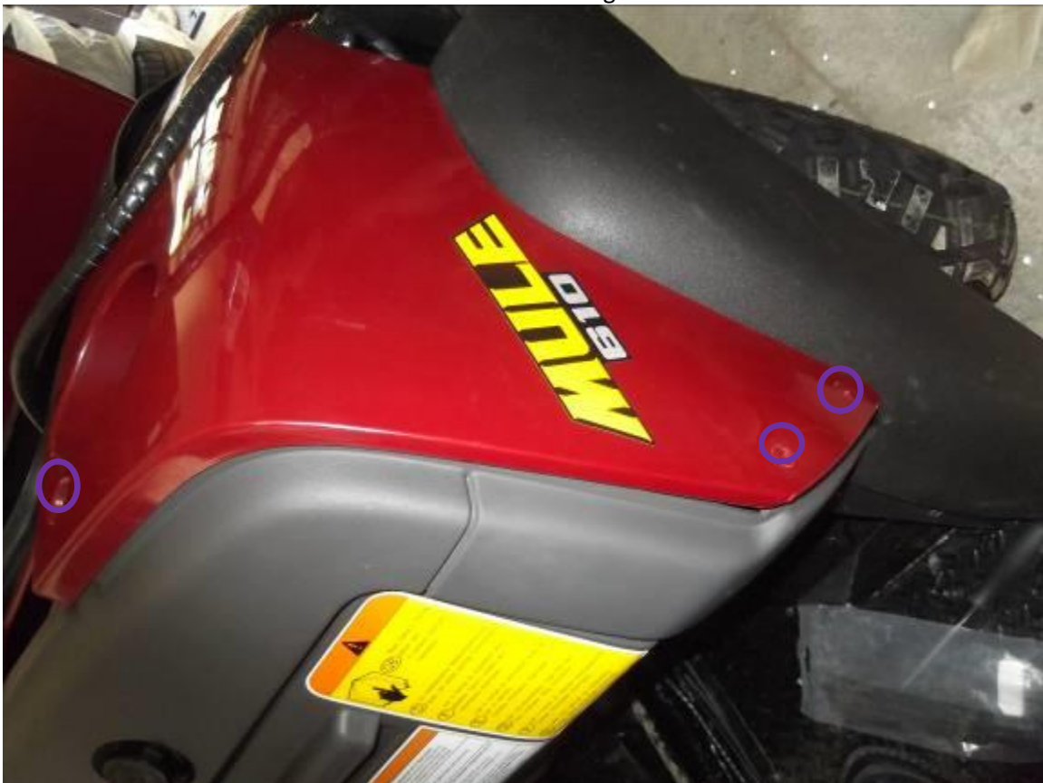
Loosen the screws on the dashboard right side and save these.
