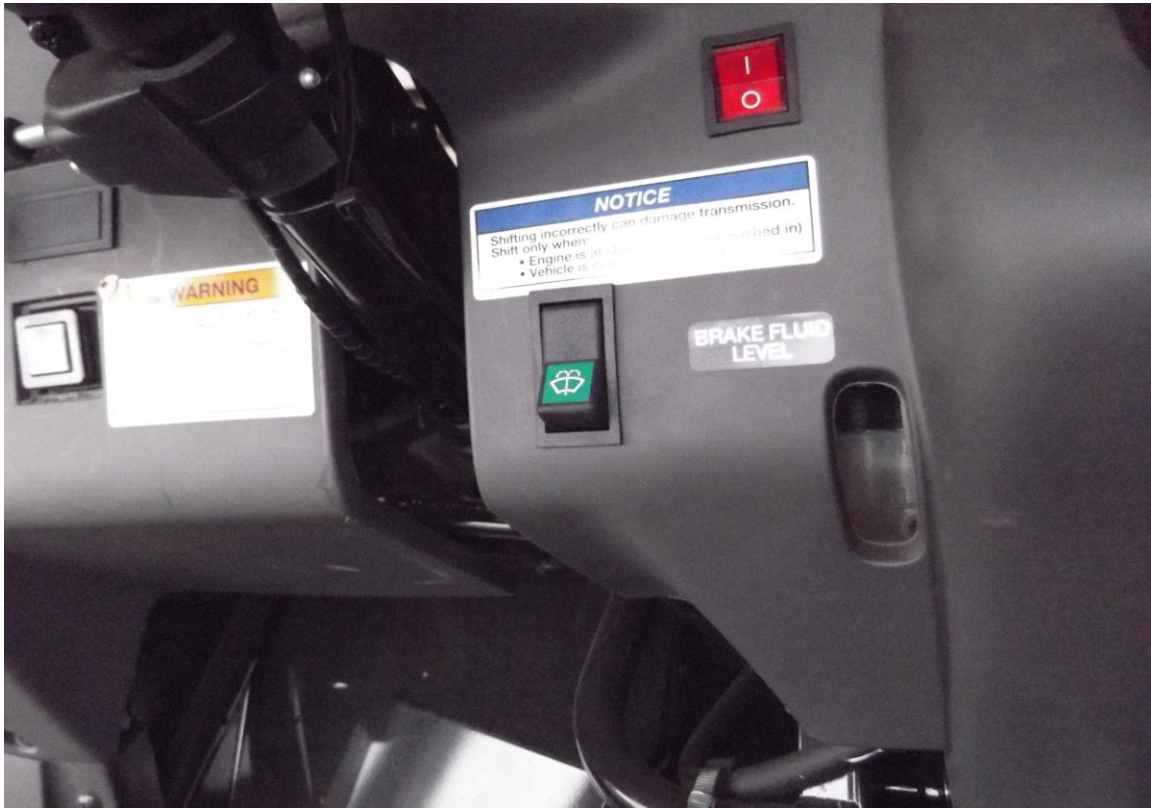
Loosen the screws on the dashboard right side and save these.
