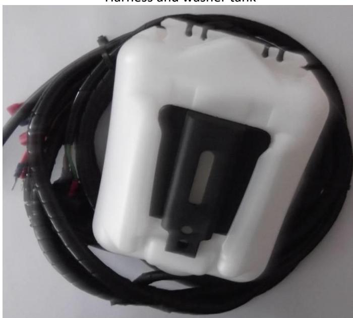
Harness and washer tank
