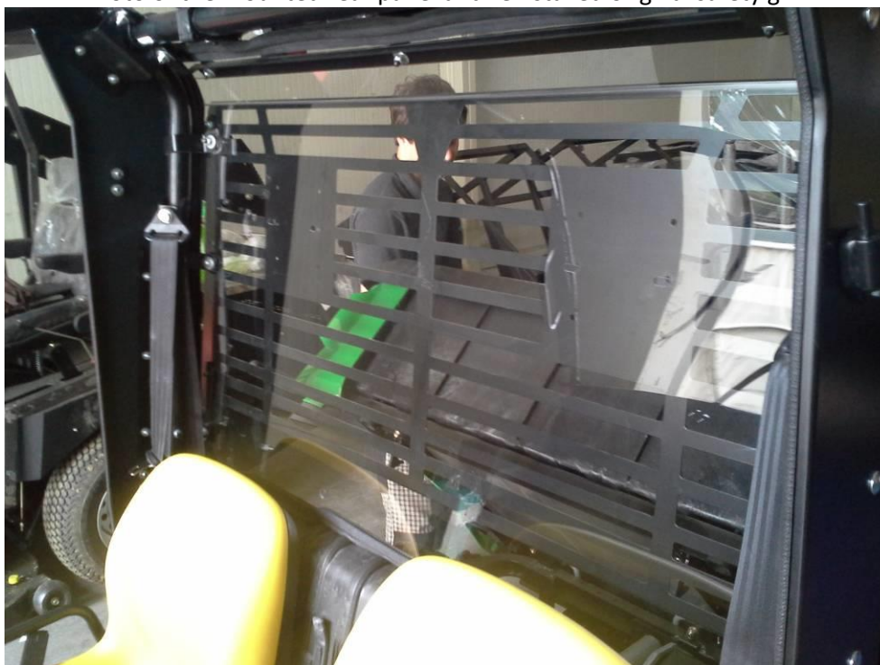
Photo of the mounted rear panel and reinstalled original safety grill.
