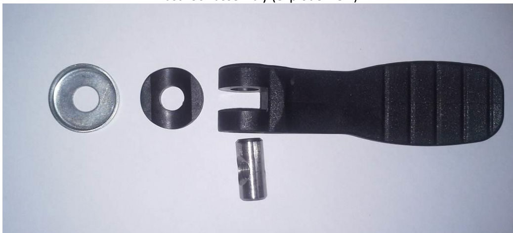
Fast-lock assembly (explode view).
