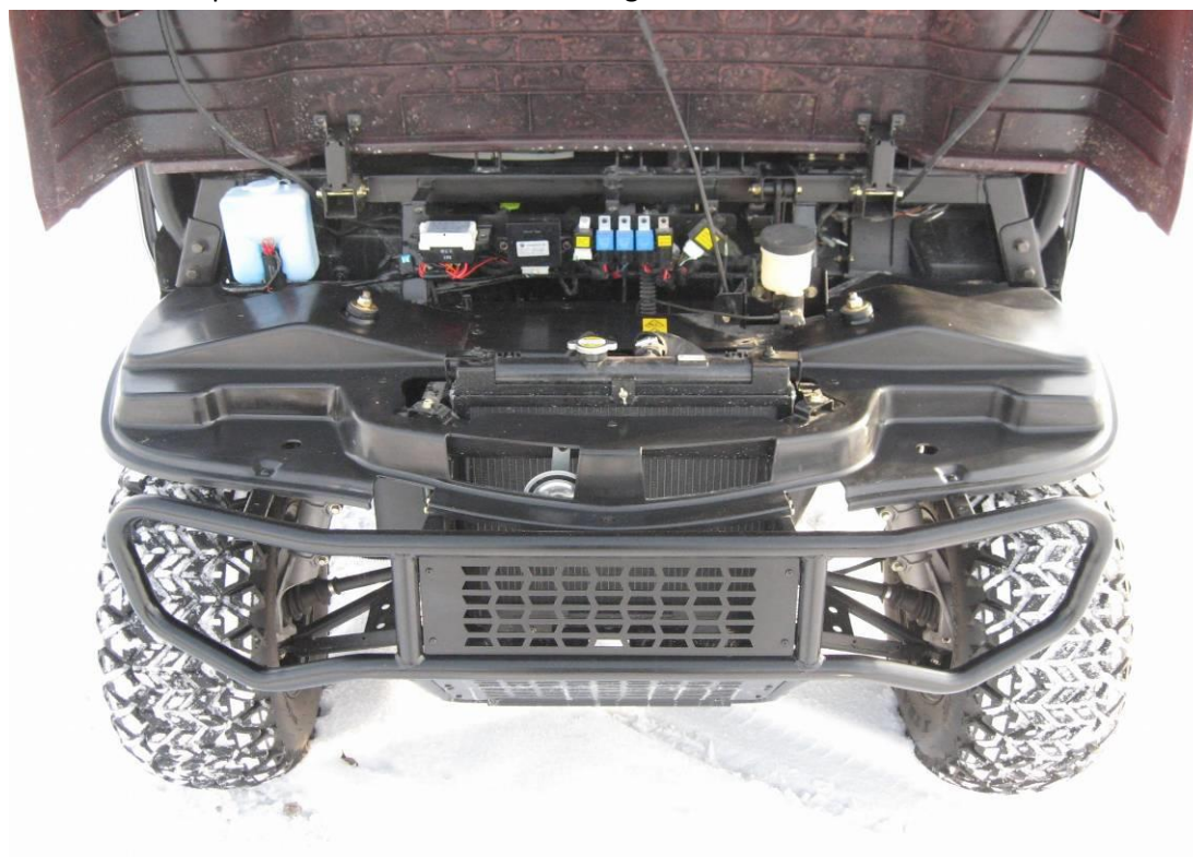
Washer tank placed in front of the cart through the bracket bolt to the truck frame.
