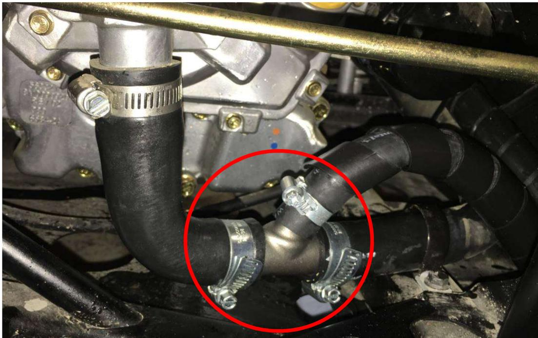
Secure the original cooling system hose with clamps and cut the hoses between the clamps (red line).
