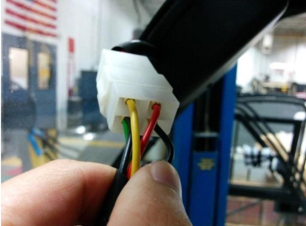
Connect the wiper/washer harness to the original electroinstallation.
