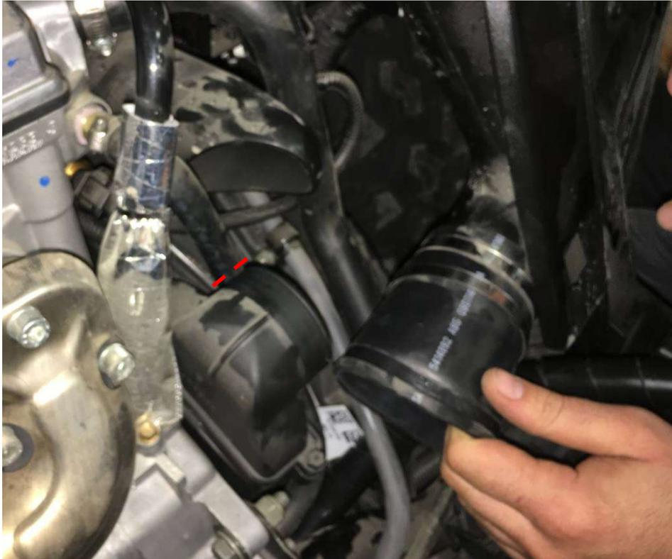
Install the "Y" coupling into the hose and fix with tightening straps. Install the heater hose onto the coupling a fix with tightening strap. Tighten hard.
