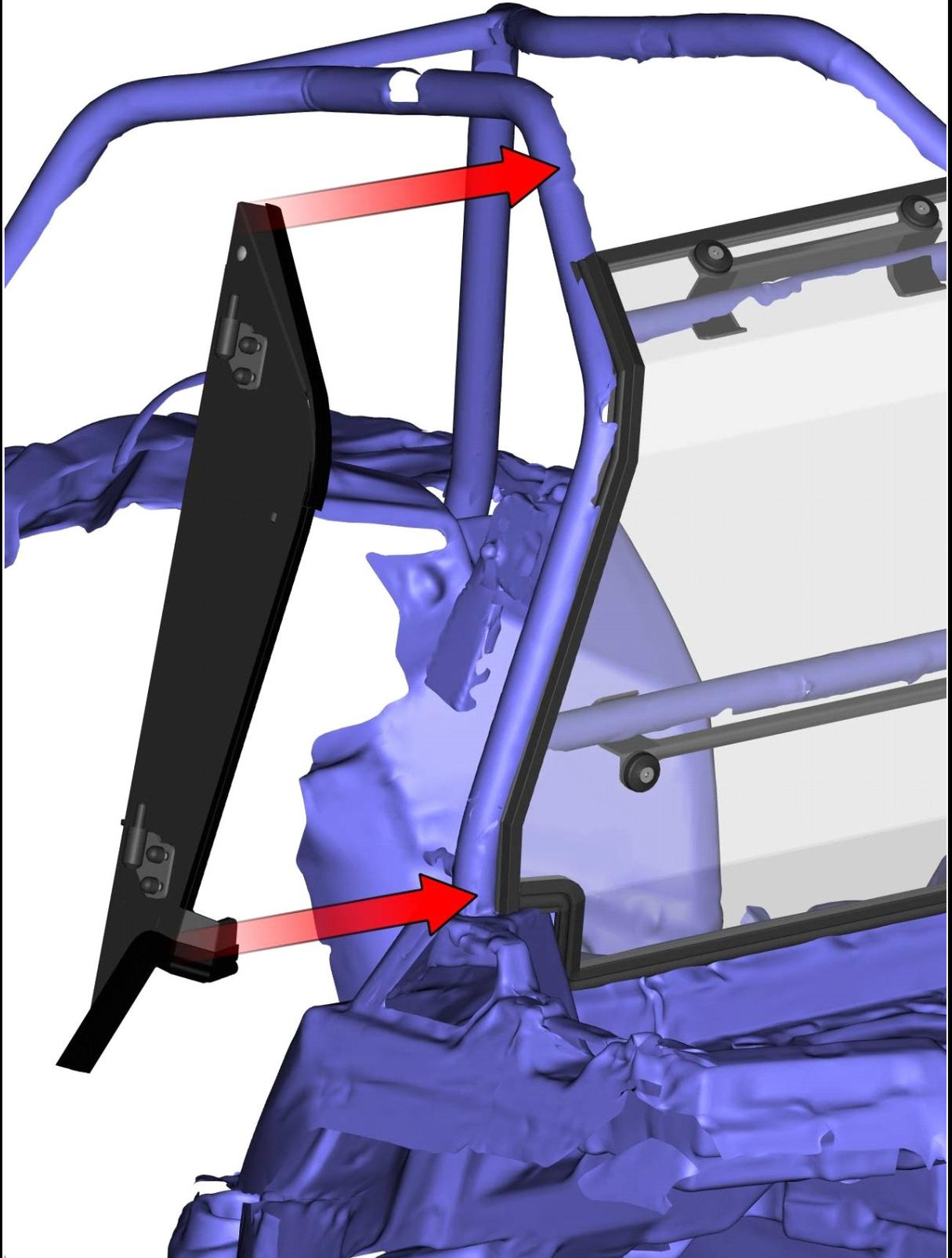
Fix the left door base with the roler cage by included fixing assemblies.
