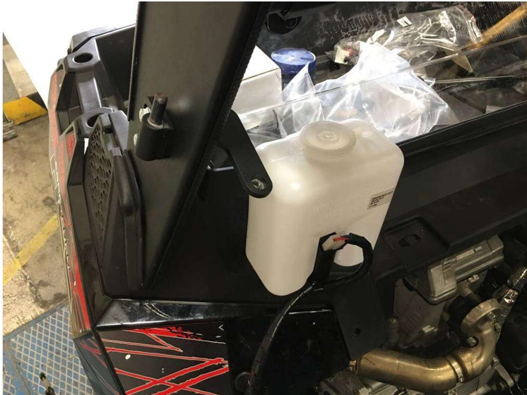
Connect the wiper and washer harness branch with the switch. Detailed view.
