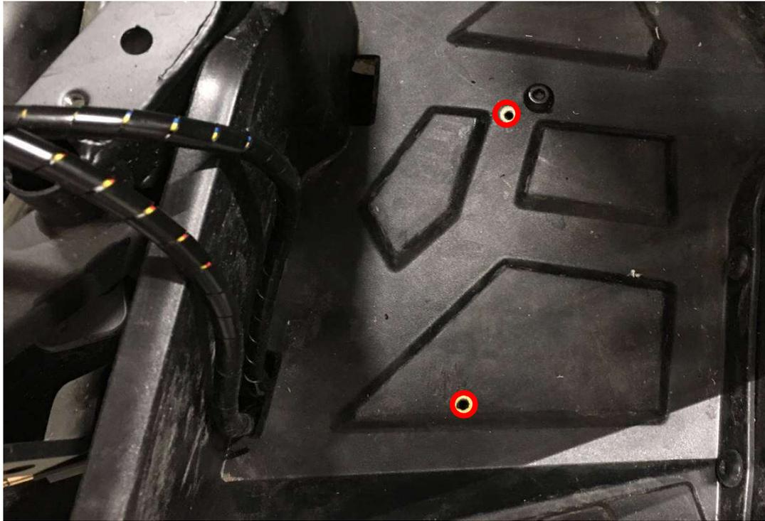
Fix heater assembly onto position with included fixing assemblies.
