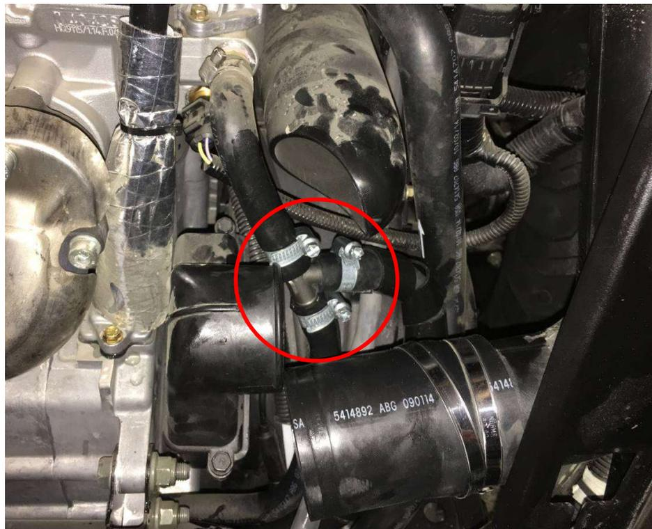
Before first use bleed air out of the cooling system. Loosen the bleed screw (red circle). Turn on the engine and let it run until the radiator bleeds out air.
