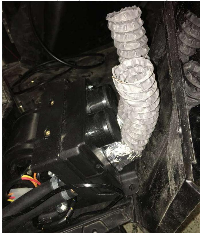
Install the water hoses and fix it with tightening straps. Tighten hard.
