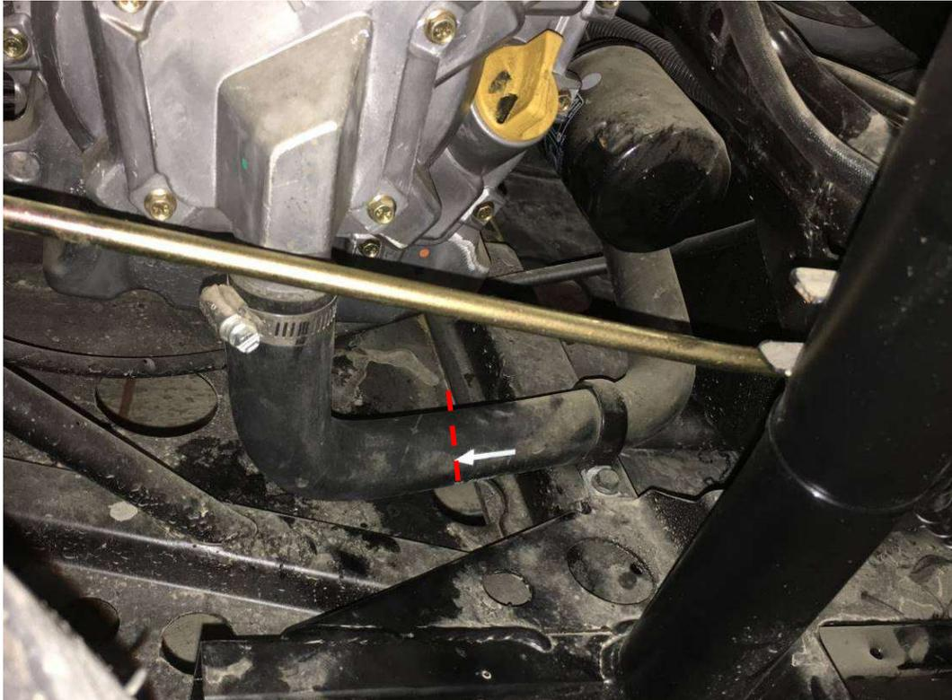
Install the "Y" coupling into the hose and fix with tightening straps. Install the heater hose onto the coupling and fix with tightening strap. Tighten hard.
