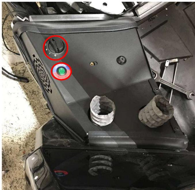
Connect the heater switch body with the harness branch. Detail view.
