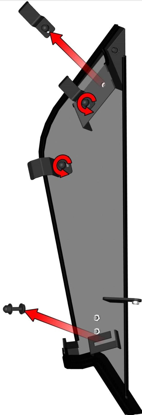
Place the door base onto roller cage and adjust to the best position.
