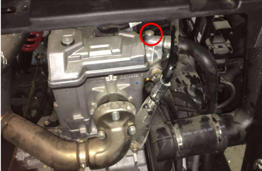
***It is absolutely necessary to bleed the air out of the UTV's engine cooling system. Incomplete bleeding of cooling system can result in engine damage. If you don't have sufficient experience with this process, we strongly recommend professional service technician assistance. We are not responsible for damages when cooling system bled incompletely. Please note that additional heater system will absorb more than 2 liters of coolant fluid.***
