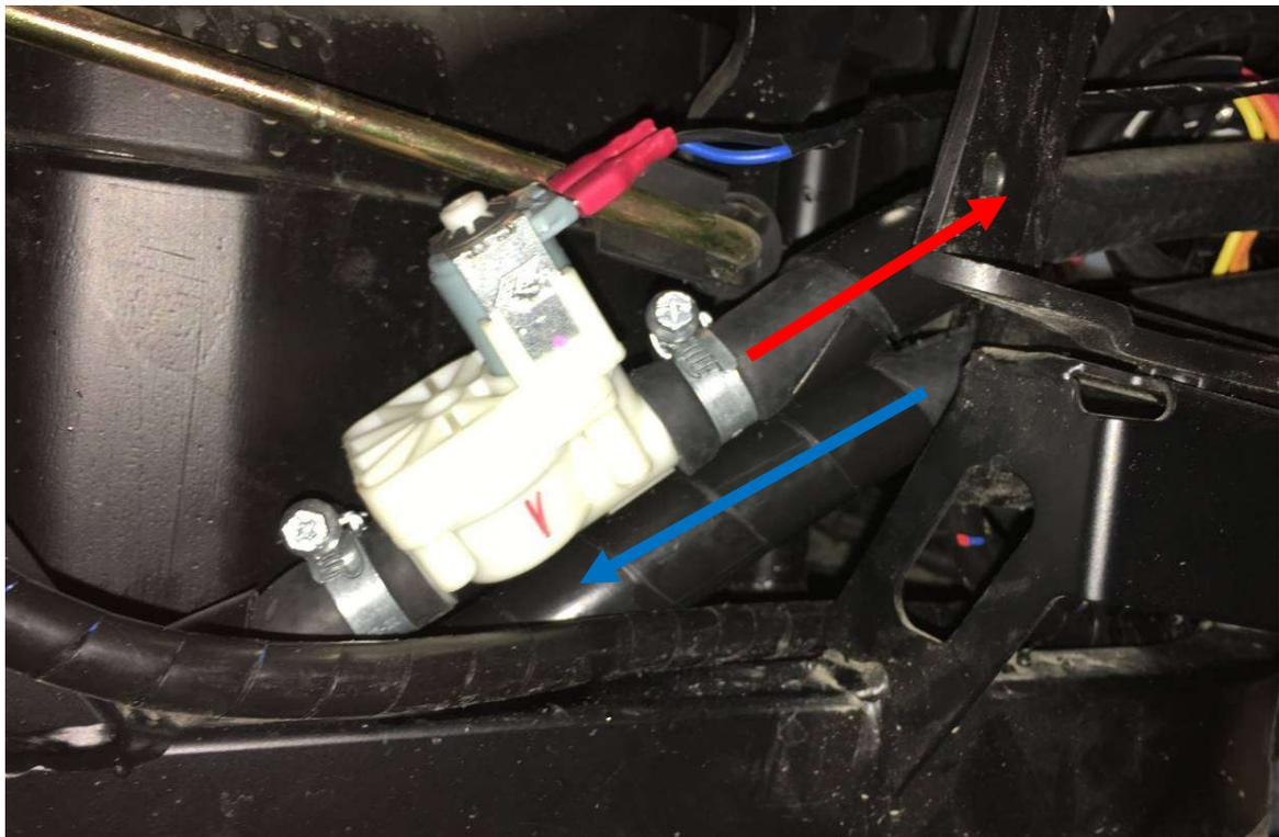
Lead the hot water hose to the engine space (red line) and the cold water hose to the cooler (blue line)
