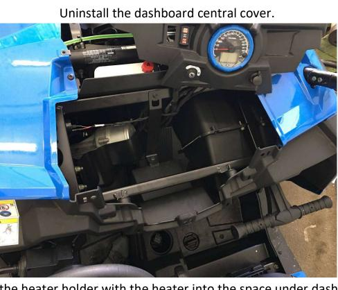
Install the heater holder with the heater into the space under dashboard central cover (red circle).
