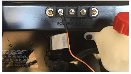
Connect the relay harnesses to the original electroinstallation.
