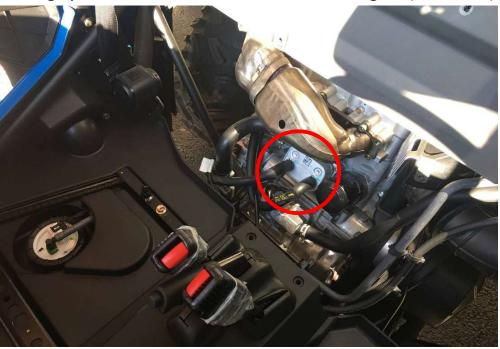
Secure the original cooling system hoses with clamps and cut the hoses between the clamps. Install the "Y" coupling into the hoses and fix with tightening straps (red circle). Tighten the straps hard.
