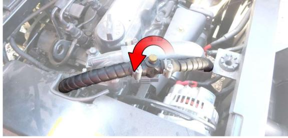
2. To achieve engine operating temperature depress the accelerator to increase The engine RPM. This will increase the preasure and flow of the water pump forcing more coolant through the heater. After operating temperature ceache turn of engine and open it. Trapped air should come out from heater system throughout bleeding valve.
