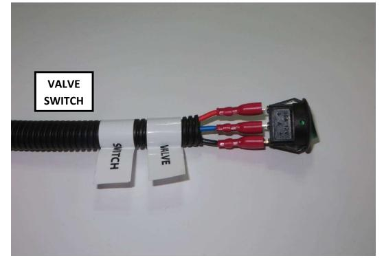
Connect the ventilator harness branch with the ventilator switch.
