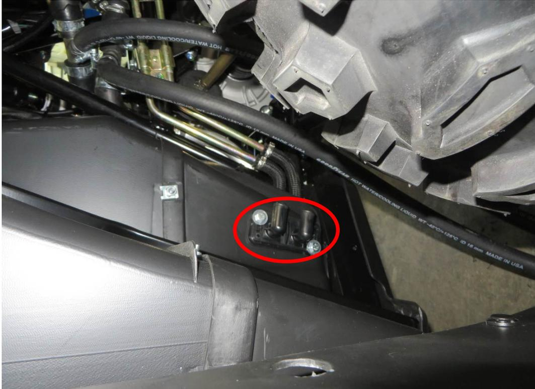
Connect the bended hoses with the heater and with the el.valve on one side and to the heater hoses pass on the other side and fix by tightening straps.
