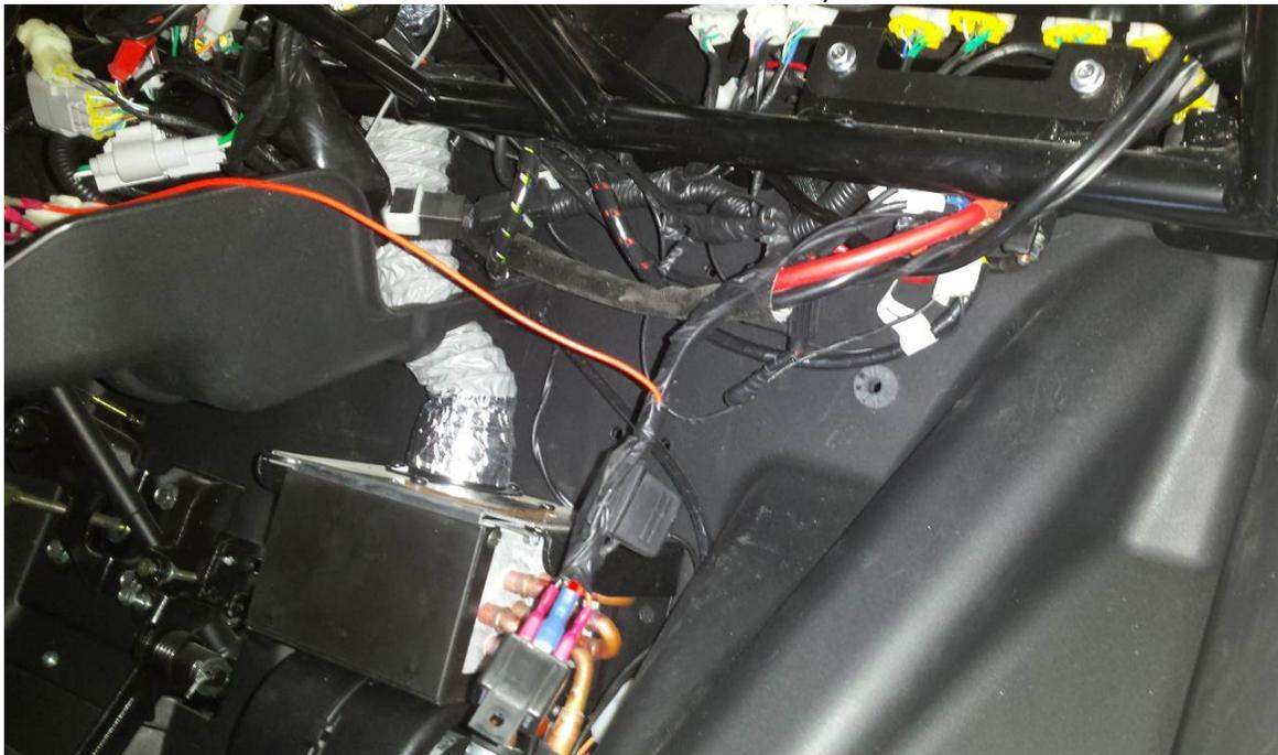
Connect the relay harness to the original electro installation (detailed view).
