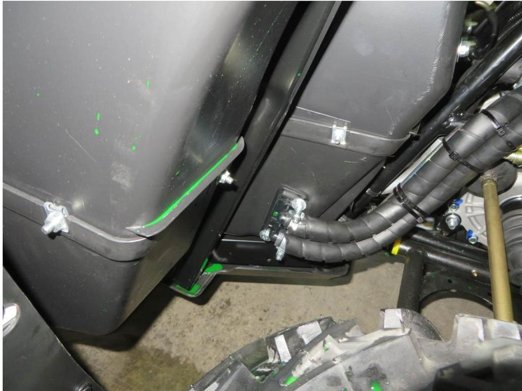
Cut the original engine cooling system hoses and insert "Y" couplings. Install the heater hoses onto the "Y" couplings. Fix both by included tightening straps.
