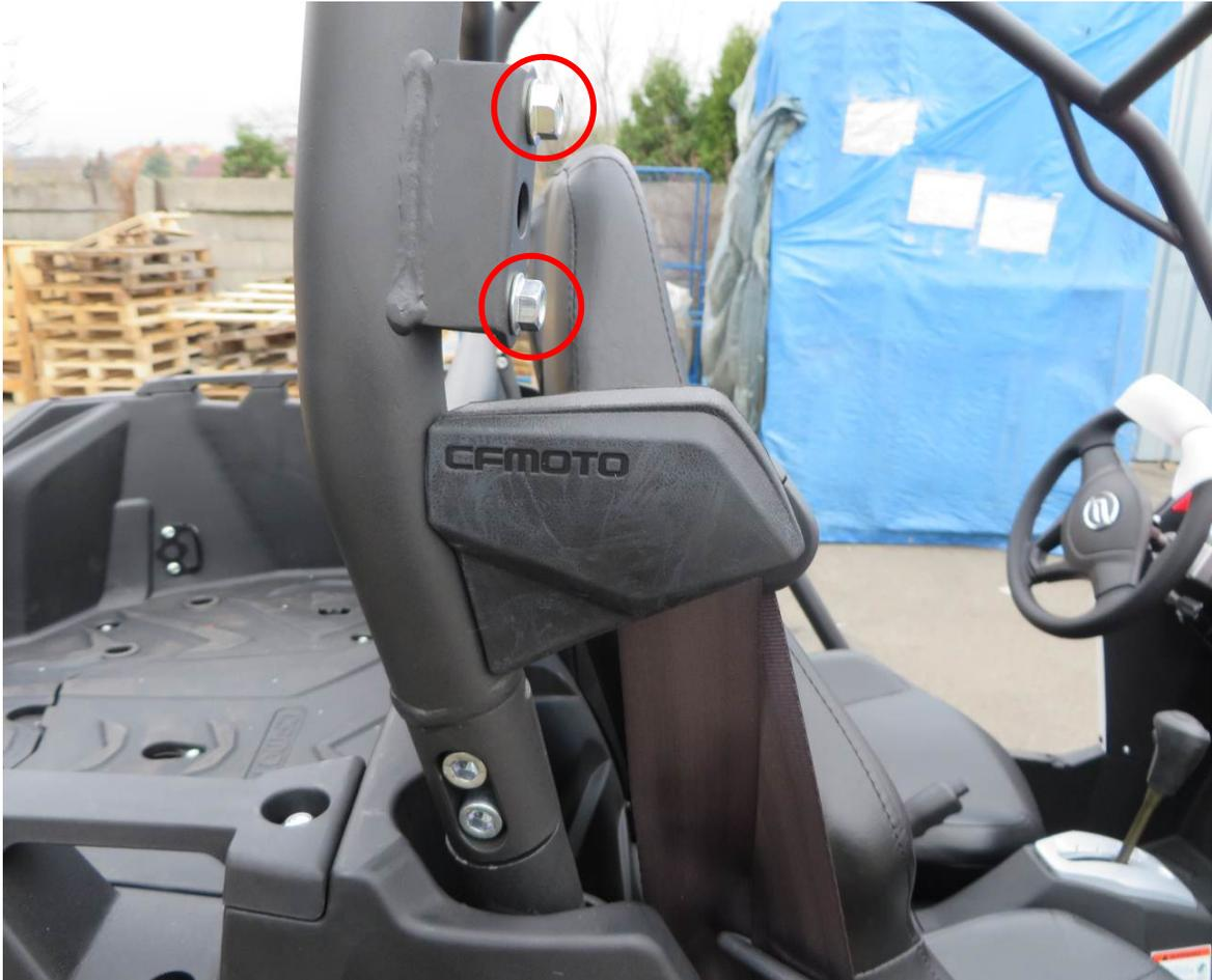
Place the left door base onto the roller cage and adjust the door base into the best position.
