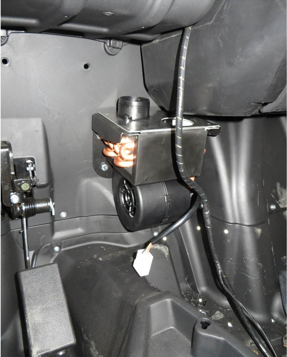
Connect the harness branch with the heater connector.
