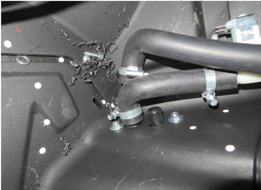
Connect the heater hoses to the heater hoses pass and fix by tightening straps.
