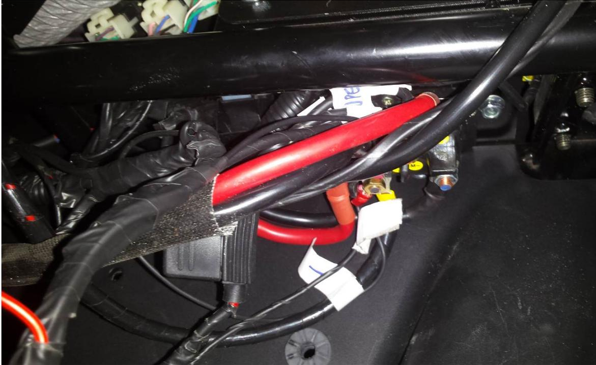
Lead the single relay harness branch to the central panel and connect it with the original electroinstalation.
