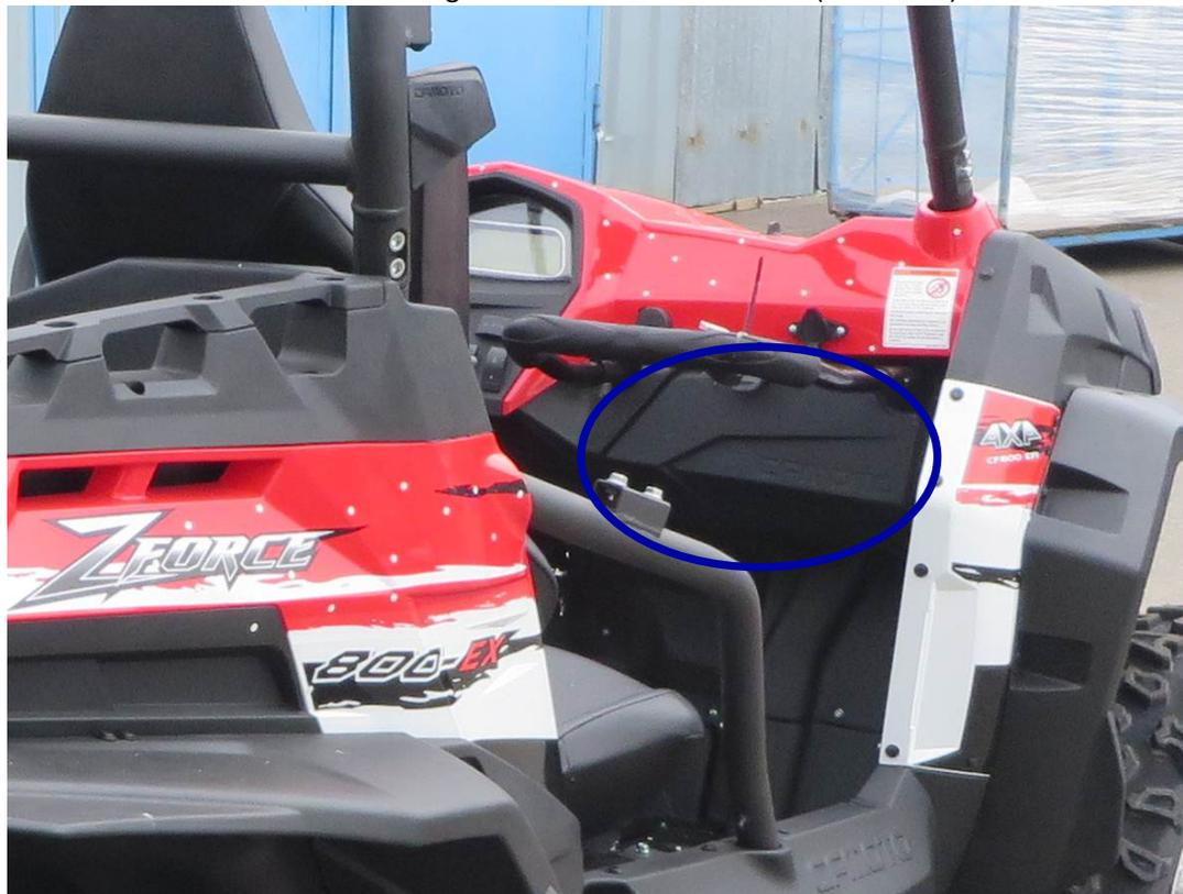
Carefully cut hole  $\varnothing 50\text{mm}$  for the air vent into the dashboard (blue circle), hole position must be chosen in order the hole have to be hidden under the air vent cover. Lead the air hose PVC through the hole.
