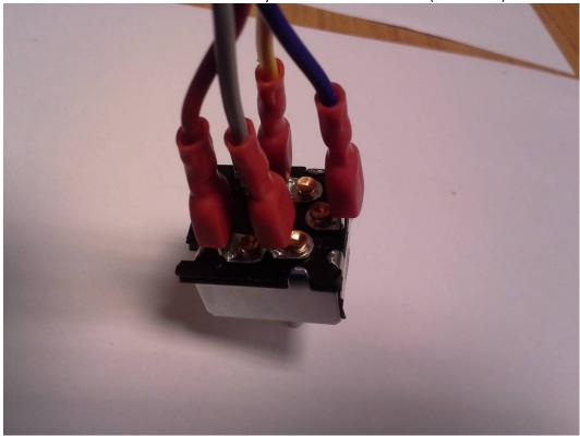
Connect the harness branch with the el.valve switch. (Detail view)
