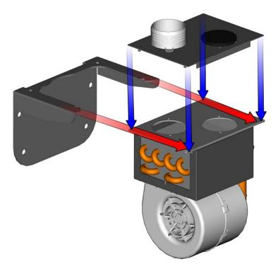
Fix the heater assembly with the heater holder by included nuts and washers.
