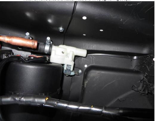
Connect the el. valve harness branch to el. valve (detailed view).
