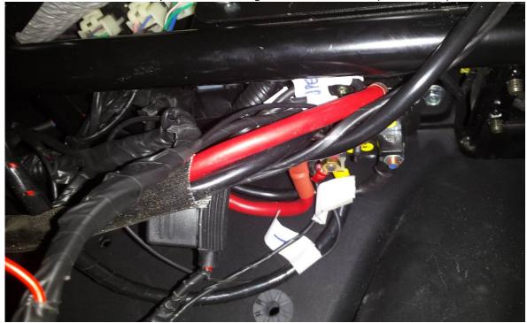
Lead the single relay harness branch to the central panel and connect it with the origingal electroinstalation.
