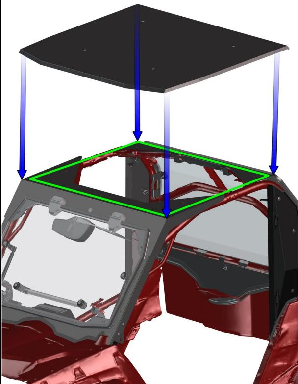
Fix the roof with the UTV rollercage by included holders, screws, nuts and washers on both sides.
