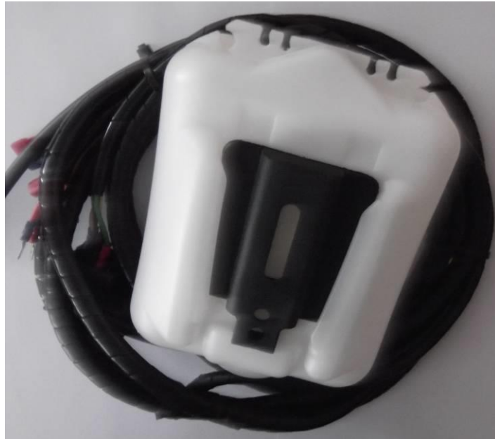
Harness and washer tank
