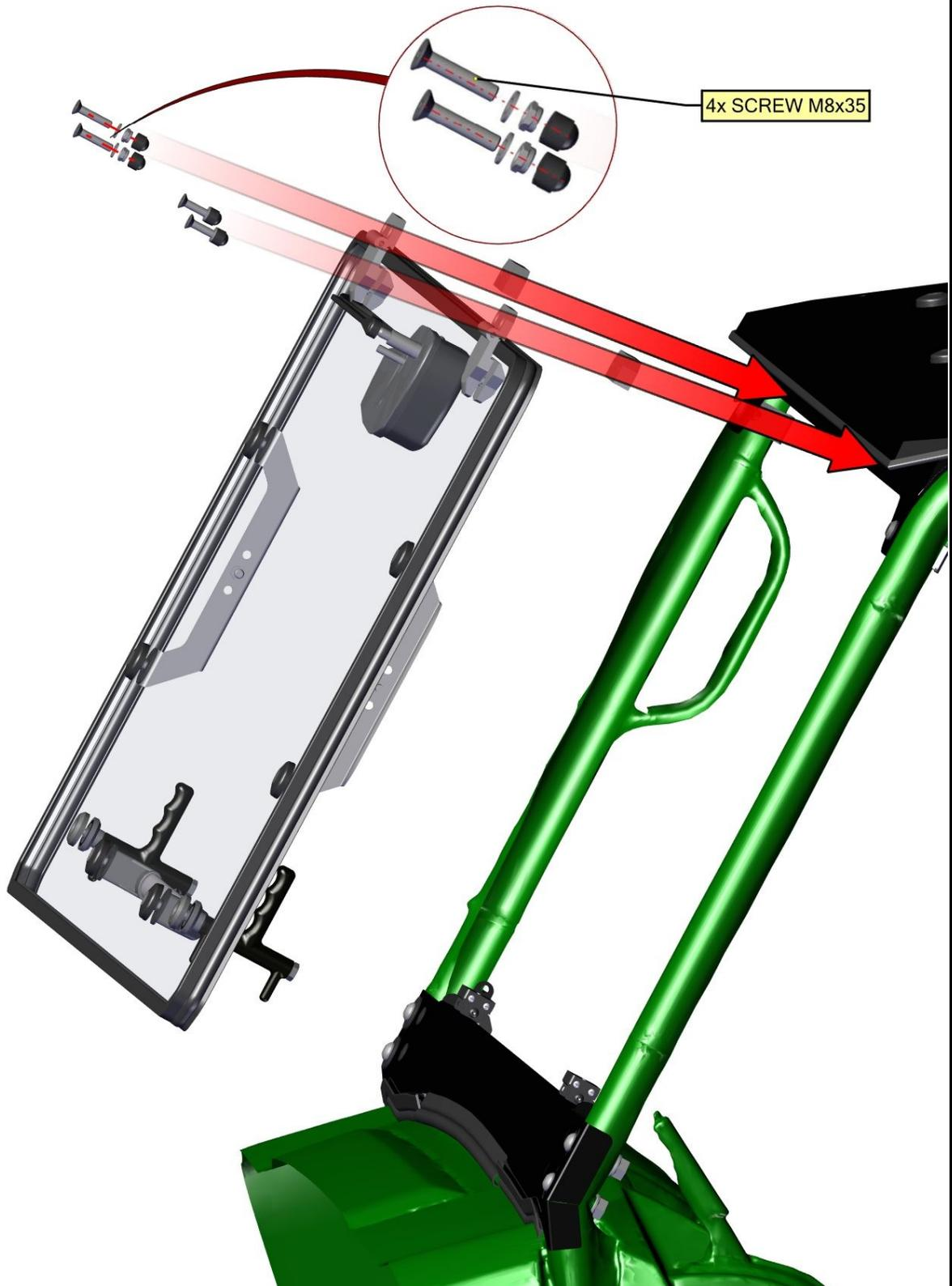
Install gas spring into the gas spring holders and fix by included self-locking nuts, washers and covers. On both sides.
