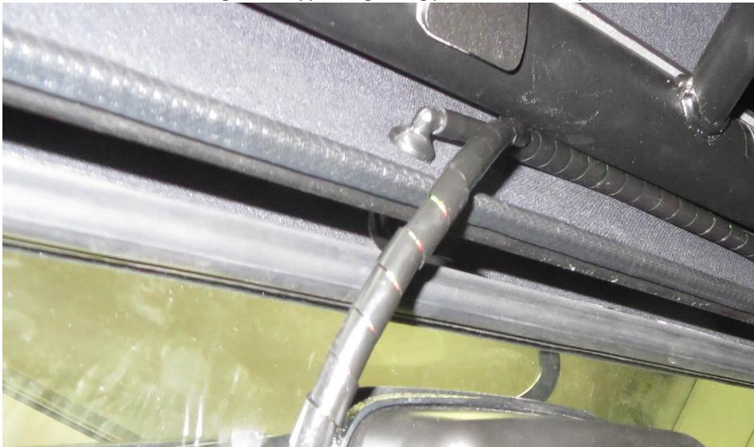
Connect the washer tube to the washer jet.
