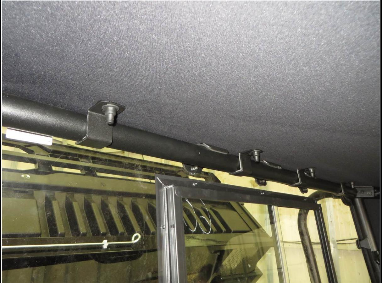
Place the front upper ledge/roof holders onto the front upper ledge and fix by included screws, washers, nuts and covers.
