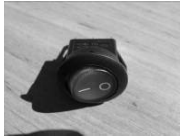
El. Vent switch
