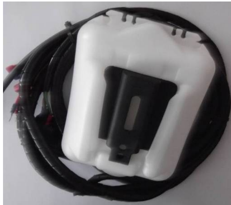
Harness and washer tank
