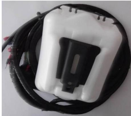
Harness and washer tank
