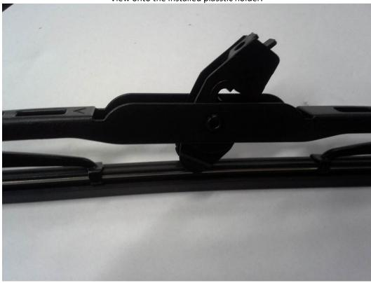
Insert the wiper arm hook onto the wiper latch plastic holder and press it into the correct position.
