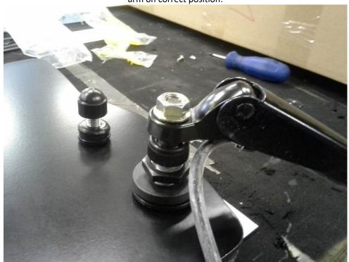
Fix the wiper arm with the wiper motor pin by included nut. Insert plastic holder onto the wiper latch pin in correct position
