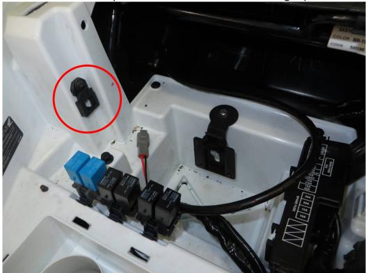
Install the relay harness onto the relay harness holder.
