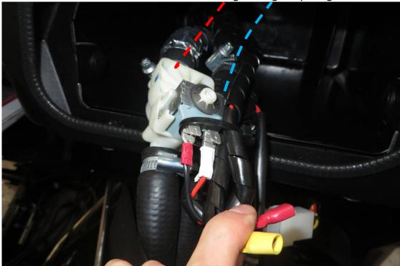
Connect the heater harness female pins with the el. valve male pins.
