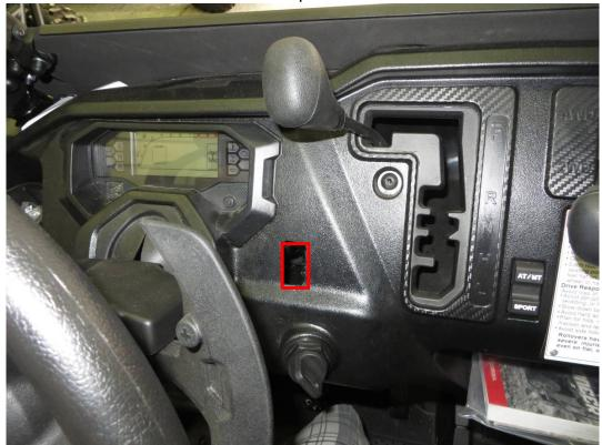
Drill holes into the glove box for the heater water hoses and heater harness.
