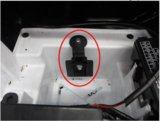
Install the washer tank onto the washer tank holder.
