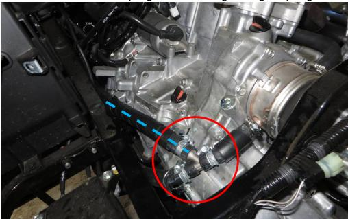
Secure the original cooling system hose with clamps and cut the hoses between the clamps. Install the "Y" coupling into the hose and fix with tightening straps. Install the heater hose onto the coupling a fix with tightening strap. Tighten hard.
