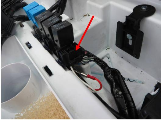
Install the relay back to the original position.
