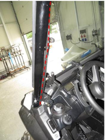
Route the wiper motor harness under the front upper ledge holder.
