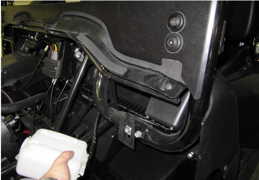
Install the washer tank onto the washer tank holder.
