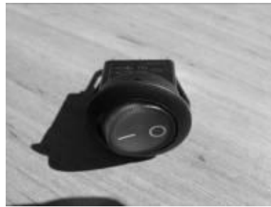
El. Vent switch
