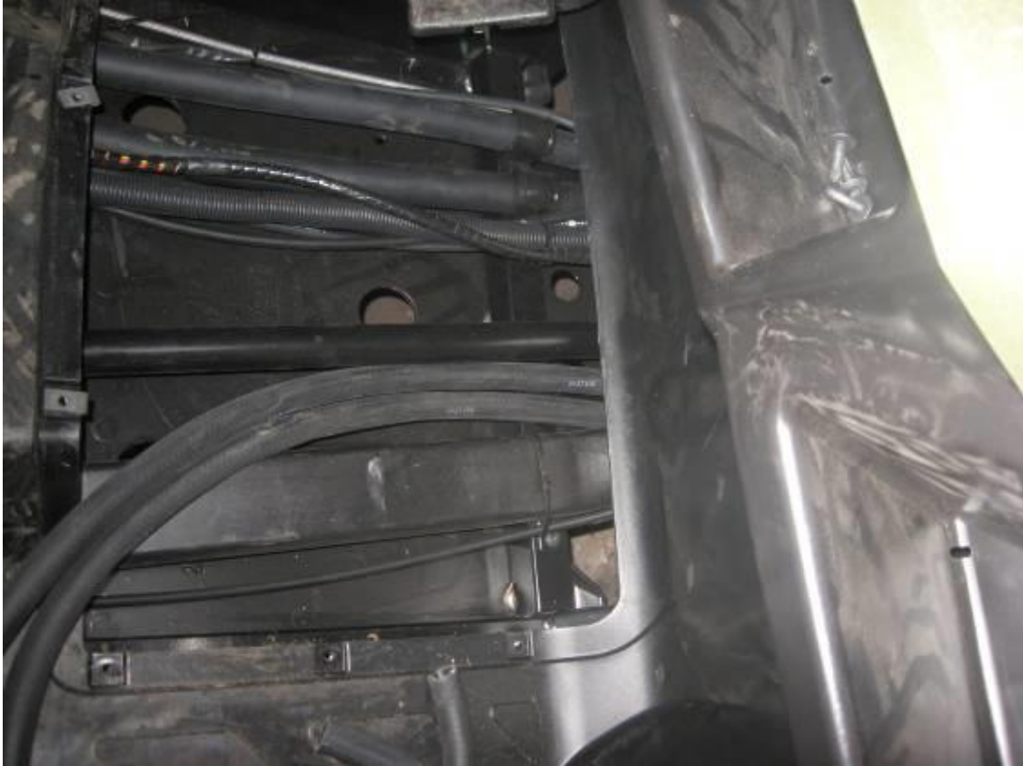
Water hoses in the floor tunnel.
