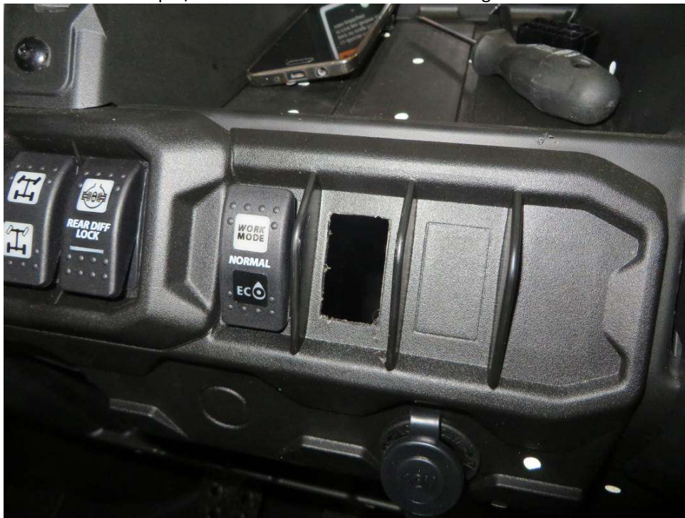
Carefully cut of the dashboard switch blank. Lead the wiper/washer switch harness branch through the dashboard.
