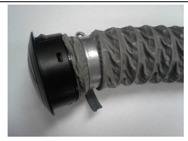
Repeat previous step with the dashboard air vents and press the vents into the dashboard.
