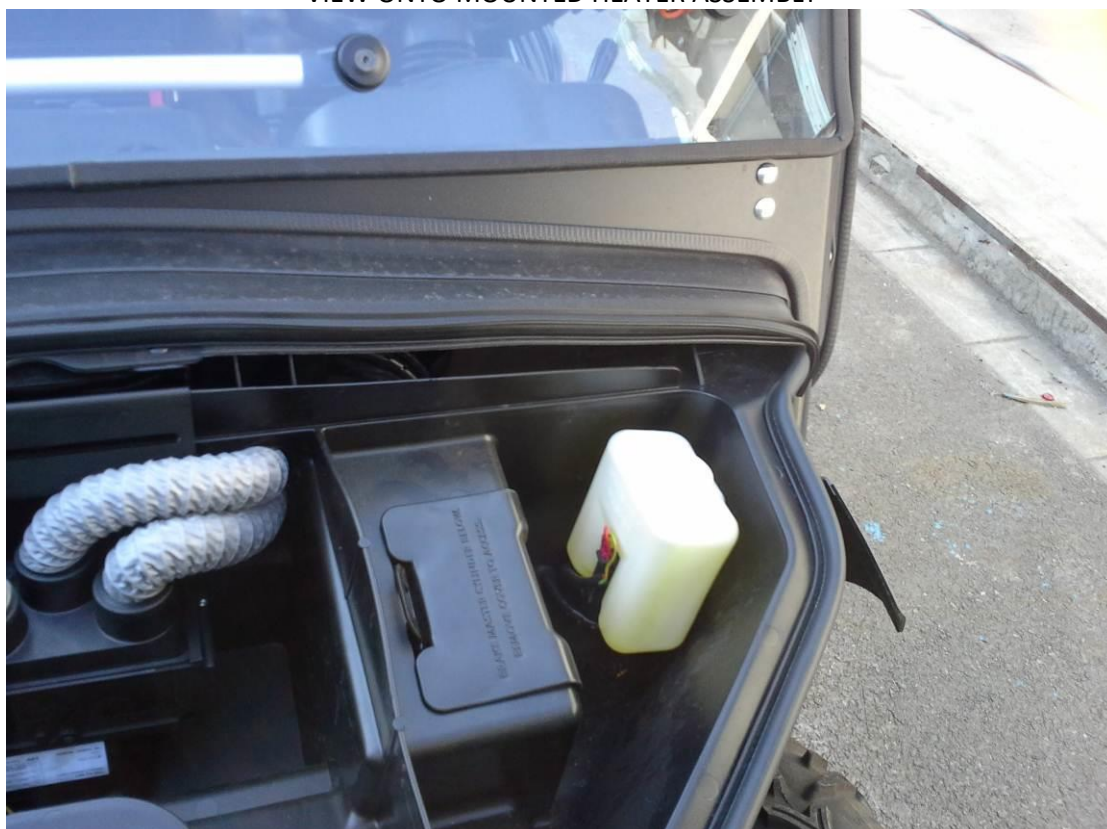
VIEW ONTO MOUNTED HEATER ASSEMBLY
