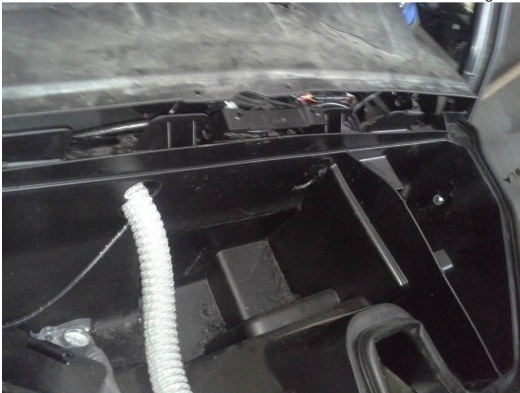
Connect the branch no.:1 with the heater connector. DETAIL VIEW
